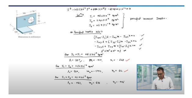
Now, this equation is in the form of  $I^3$ . Therefore, it will have three solutions of the I's and let me write down the solution. So  $I_1=48.3\times 10^{-4}~kg~m^2$ .  $I_2=11.82\times 10^{-4}~kg~m^2$  And  $I_3=43.4\times 10^{-4}~kg~m^2$ .
