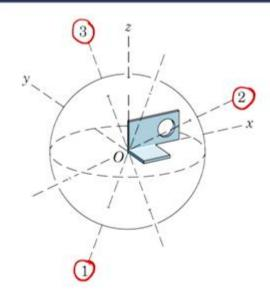
And similarly, for  $I_i = I_3 = 43.4 \times 10^{-4} \, kg \, m^2$ .  $l_3 = 0.0183$ ,  $m_3 = 0.895$ , and  $n_3 = 0.445$ . So, these are the direction cosines of the principal inertia axis. Now, let me show you the orientation of the principal axis of inertia corresponding to  $l_1$ ,  $m_1$ , and  $n_1$  we have the first principal axis.
