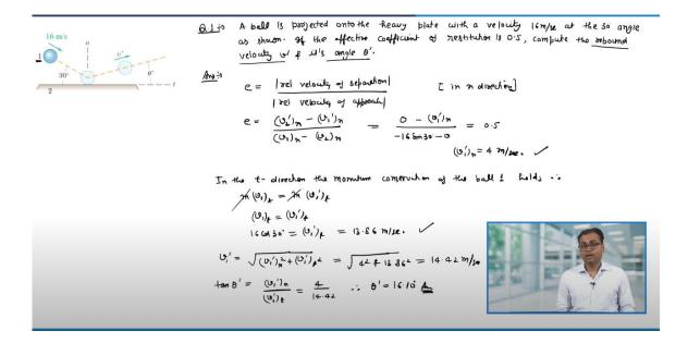
Now, let us look at some of the examples based on this concept. This is the first problem statement. A ball is projected onto the heavy plate with a velocity of 16 m/s. At the 30° angle as shown. If the effective coefficient of restitution is 0.5, compute the rebound velocity v' and its angle  $\theta'$ . So, clearly, this is the example of oblique angle impact, and we have to find out what is the rebound velocity v' and what is the rebound velocity v' and what is the rebound velocity v' and v'.
