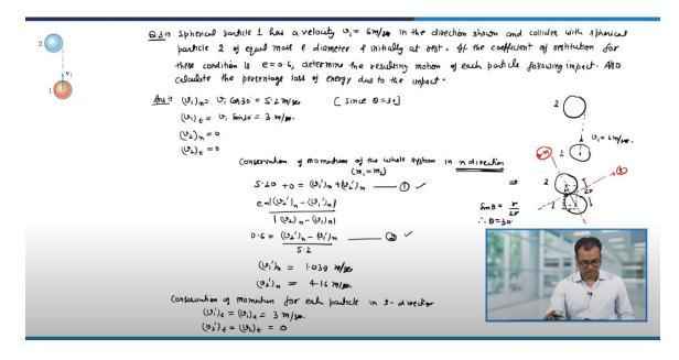
Now, let us look at another problem statement. A spherical particle 1 has a velocity  $v_1 = 6 m/s$  in the direction shown and collides with a spherical particle 2 of equal mass and diameter and initially at rest. If the coefficient of restitution for these condition is e = 0.6 determine the resulting motion of each particle following impact. Also calculate the percentage loss of energy due to the impact.
