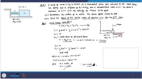
Now, let us look at the another problem statement. A block of mass 1.6 kg is placed on a horizontal plane and attached to an ideal spring. The spring has a stiffness of k = 30 N/m
