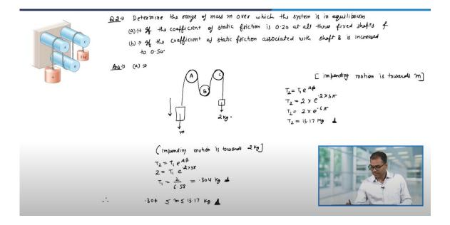
Let us look at one more problem on the similar concept and the problem statement is following. Determine the range of mass m over which the system is in equilibrium (a) if the coefficient of static friction is 0.20 at all three fixed shafts and (b) if the coefficient of static friction associated with shaft B is increased to 0.50.
