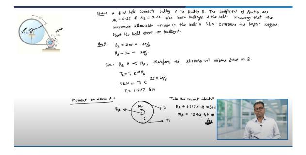
Now, the radius of the pulley A is 8 inch which can be written as 200 mm and the radius of pulley B is 1 inch which is 25 mm. So, again you can use the same concept since  $\beta_B$  is less than  $\beta_A$ . Therefore, the slippage or the slipping will impend first on B.
