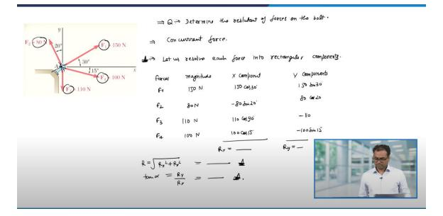
So, herein, there are four forces which are acting on a bolt. And the question statement is, determine the resultant of the forces on the book. So, you can see here there are four forces, their magnitudes and direction is given and the question is can we reduce this force system into a single force. So, first thing we have to see here that the forces are concurrent because their line of action they meet at a single point.
