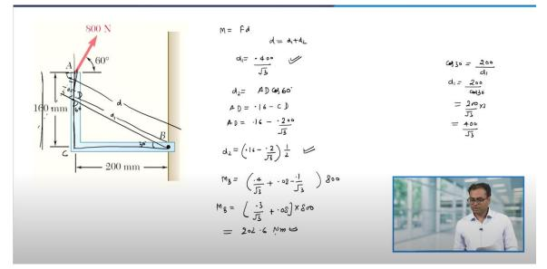
So, let us use that method and let us see if the answer is same using M = Fd where this d is the perpendicular distance from B to the force. Now, force is a sliding vector. So, therefore, we can slide it and we can draw a perpendicular. So, this is d and this i can write down as  $d_1$  and this i can write down as  $d_2$ . So, d becomes  $d_1 + d_2$ .
