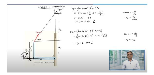
We can also calculate the moment of this force using the principle of transmissibility. So, let us slide it along its line of action. So, we have slided it on the horizontal axis. So, this is the force 800 N and this angle is 60°. Now, the moment about B will be this force we can break into the x and y component. So, the x component will not contribute because its moment about B will be 0. So, the only moment that is going to contribute is the y component of the force.
