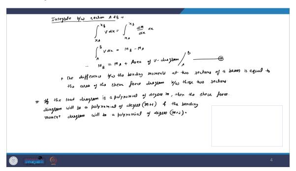
Now, to find out what is the value of M, let us again integrate this between A and B. So, let us integrate between section A and B. So,  $\int_{x_A}^{x_B} V dx = -\int_{x_A}^{x_B} \frac{dM}{dx} dx$ . So, this gives you  $\int_{A}^{B} V dx = M_B - M_A$  or we can write down  $M_B = M_A + \text{Area of V-diagram}|_{B}^{A}$ . Let us call this equation number 4 and we can again write it down in the text. This implies that the
