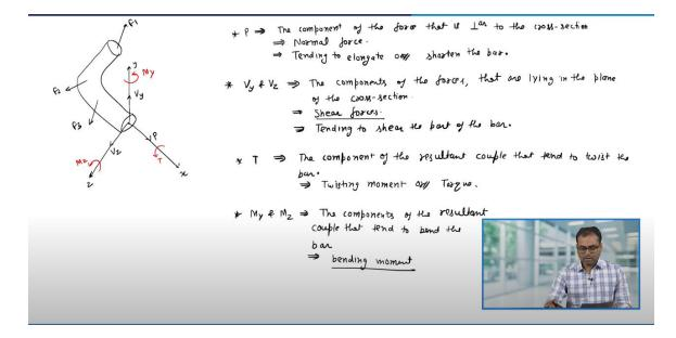
It has a tendency to elongate or shorten the bar. Now, let us look at what is  $V_y$  and  $V_z$ . So, this is the component of the forces that are lying in the plane of the cross-section. And these forces are called the shear forces. And they have a tendency to shear the part of the bar. Now, we have couple T. This T is the component of the resultant couple that tend to twist the bar.
