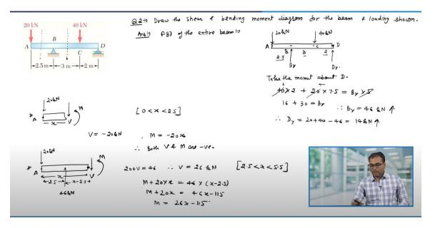
Here, the problem statement is following. Draw the shear and bending moment diagram for the beam and loading shown okay. So, as we did first, let us find out the reaction forces and for that, let us consider the free body diagram of the entire beam.
