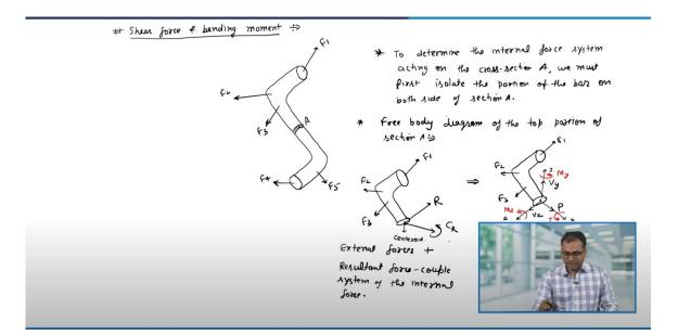
Today, we are going to learn that if the external forces in a member is given, then we can also calculate the internal forces by the analysis of equilibrium. Now, these forces are particularly the shear force and the bending moments. So, let us understand what is shear force and the bending moment.
