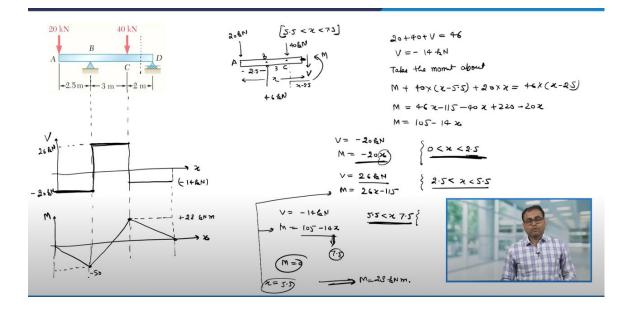
To find out the shear forces and bending moment, let us first cut the beam between A and B. So, we are interested first in the region wherein x is between 0 and 2.5.
