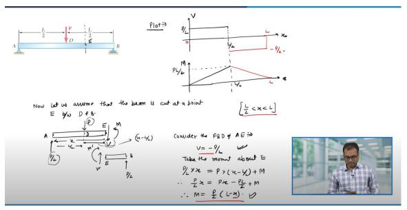
So, therefore, both the shear and the bending moments are positive. Now, let me plot this. So, let me first plot the shear force. So, this is x and just now we have calculated that the value of the shear force is P/2. So, it is independent of x and we have calculated this in the region between 0 and L/2.
