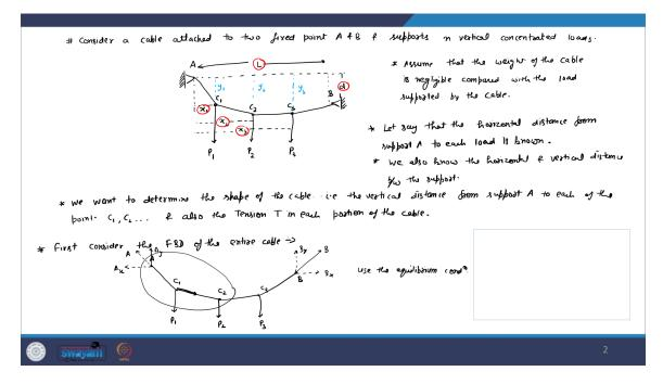
Let us consider a cable that is attached to let's say two fixed point, let us call them A and B and this cable supports let's say n vertical concentrated loads. And as we assumed previously, let's say this cable is flexible and also its weight is negligible compared to the weight of the load. So, we have let's say these two fixed points, let us call them A and let's say B and this cable is hanging between A and B and there are n number of concentrated loads.
