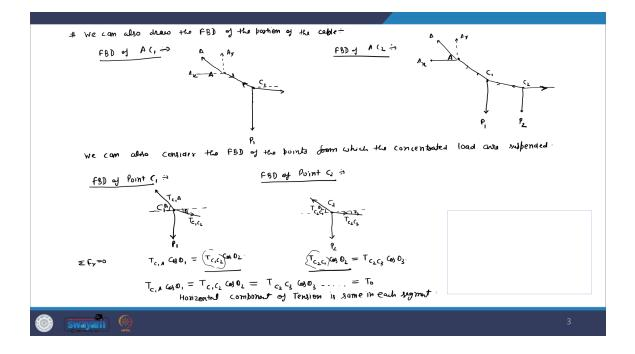
So, therefore, its part is also in the equilibrium. So, what I can do is, let us consider the free body diagram. So, as I said, we can also draw the free body diagram of the portion of the cable. So, let's say that I want to draw the free body diagram of  $AC_1$ . So, I have to see what are the forces that are acting. So, let's say free body diagram of  $AC_1$ . So, this is point A and this is point  $C_1$ . So, at A, there will be force. So, look at this.
