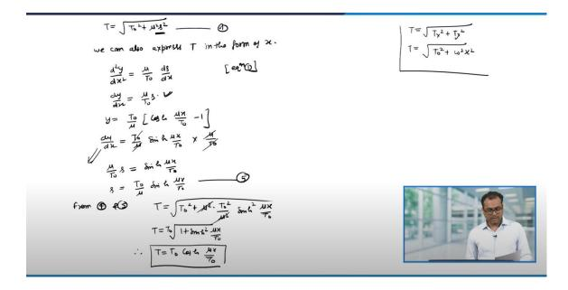
Now, let us find out the tension in the cable. When we calculate the tension, we said  $T = T_x^2 + T_y^2$  and in the previous case, it was  $T_x$  was constant because it was along the horizontal direction. So, it was  $T_0^2$  and  $T_y$  was  $w^2x^2$ . So, same as earlier, in this case, T will be  $\sqrt{T_0^2 + \mu^2 s^2}$ .
