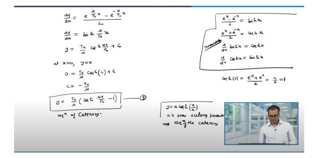
Or i can write down  $\frac{dy}{dx}$  as  $\frac{e^{\frac{\mu}{T_0}x} - e^{-\frac{\mu}{T_0}x}}{2}$  Now, this is in the form of  $\frac{e^{x} - e^{-x}}{2}$  and this function is called the *sinh* function.
