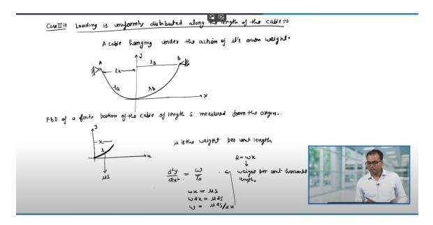
Now, let us discuss the second case where the loading is uniformly distributed along the length of the cable. So, this is case second. Here, the loading is uniformly distributed along the length of the cable. For example, you can think of a cable which is hanging under the action of its own weight. So, let us say I have a cable and this cable as I said is hanging under its own weight.
