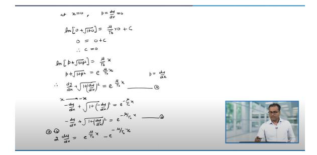
Now, to determine C, let us look at the boundary condition. So, you can see here at x = 0, my dy/dx or the slope is also 0 and  $\frac{dy}{dx} = p$ . Therefore, p will be 0. Let us use that to find out C. So, at x = 0, we have p which is nothing but dy/dx that will be 0.
