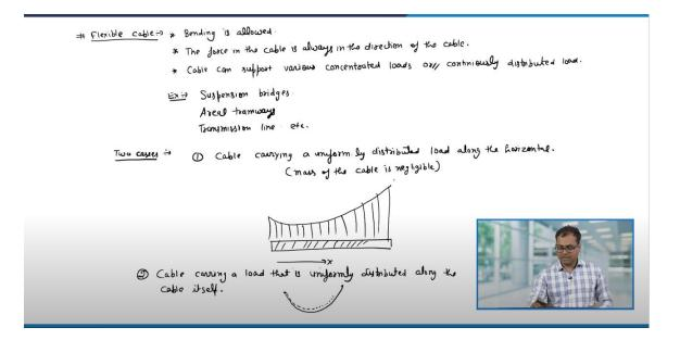
Today, we are going to talk about the flexible cable. Now, these cables can also support various kinds of loads. For example, it can be a distributed load or it can be a continuous load.
