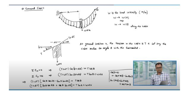
Now to analyze this, let us start with a general case. So let us say I have a cable and this cable is hanged between these two points and let us say on this cable there are some non-uniform load which is applied.
