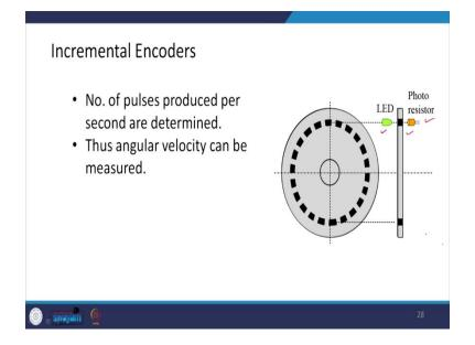
Here we have talked the principle of the encoders. We have a slotted disc here, there is a LED and there is a photo resistor over here. So, we can count the number of pulses per second and then from that, you can calculate the angular velocity.
