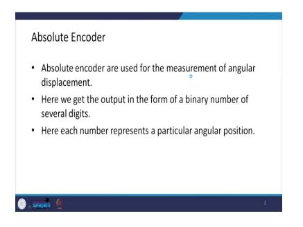
Or this is the one which I am going to talk about. Here we get output in the form of binary number of several digits and here each number actually represents a particular angular position and that is how we measure the angular displacement.
