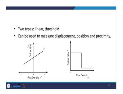
This is the type of characteristic which we can get for the linear, that is the flux density; there is a plot between flux density and the  $V_H$  that is the output voltage, it is linear. The threshold characteristic looks like this. After a certain value, there is going to be a fall in the output.
