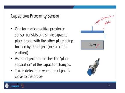
The next type of sensor is a capacitive proximity sensor. Now, one form of capacitive proximity sensor consists of a single capacitor plate probe with the other plate being
