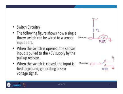
This figure shows how a single throw switch can be wired to a sensor input port. Here you can see that, this is switch single pole single throw, and when the switch is open as it is shown over here the sensor input is pulled to plus 5-volt supply by the pull up resistor. When the switch is closed the input tied to the ground generating a zero voltage signal.
