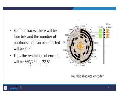
For example, in this one, you have 1111, then again 1110 and so on. For a four track as I was telling you, there will be four bits and the number of positions that can be detected will be 2 to the power 4 and this 2 to the power 4 positions will be around all these 360 degree.
