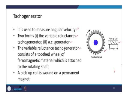
Tachogenerator is also used to measure the angular velocity. There are two basic forms available, one is the variable reluctance tachogenerator and another is the AC generator. In case of variable reluctance tachogenerator, consist of basically a toothed wheel as you can see over here of ferromagnetic material, which is attached to the rotating shaft over here. There is a pickup coil is wound on a permanent magnet.
