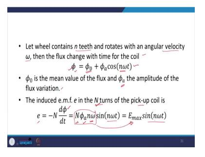
We can find out an expression over here. Suppose the wheel contains is having n number of teeth and that wheel rotates with the angular velocity  $\omega$ , then the flux change with time for the coil can be given by,
