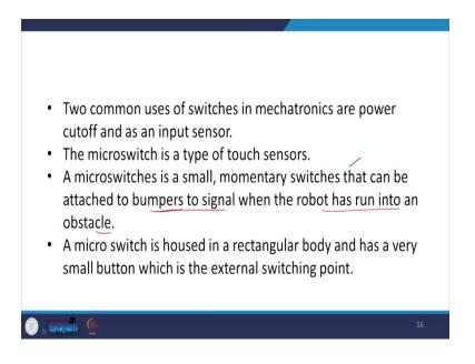
Now, two common uses of switches in the mechatronics are for the power cutoff and as an input sensor. The micro switch is a common type of touch sensor and which can be used in a small legged robot. If your robot touches some unknown obstacle then the presence of that obstacle can be detected.
