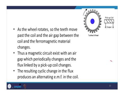
As the wheel rotates, the teeth move past the coil and the air gap between the coil and the ferromagnetic material changes. Thus, a magnetic circuit exists with air gap which periodically changes and the flux linked by the pick-up coil changes and the resulting cyclic changes in the flux produced, it produces an alternating **emf** that is electromotive force in the coil.
