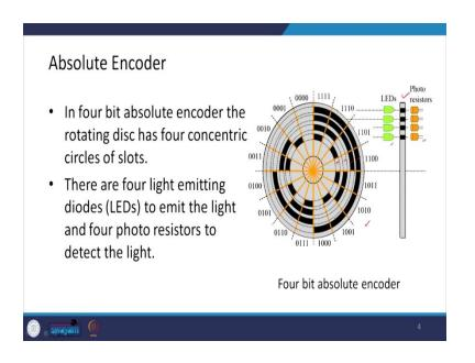
Here in the schematic, suppose there is a disc with holes are there indicated in the side view over here. There are four LEDs this side and there are four photo resistors to sense these LEDs light at the other side.
