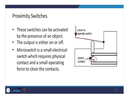
Next let us see the proximity switches. These switches can be activated by the pressure of an object. Here you can see that, the switch contact and to activate this contact we have arrangement like this and there is a lever and we can apply a force here to in order to operate the switch. The output is either on or off in this case and as I said, micro switch is a small electrical switch which require physical contact and a small operating force to close the contact.
