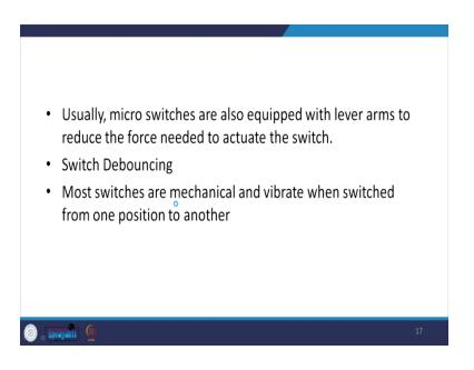
Usually, micro switches are also equipped with lever arms to reduce the force needed to actuate the switch. It is a simple mechanism if we want to amplify the forces.
