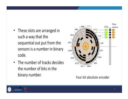
So, now these slots are arranged in such a way that the sequential output from the sensor is a number in the binary code and the number of tracks decide the number of bits in the binary code.
