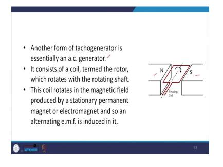
Second form of the tachogenerator is essentially an AC generator. The principle for this is simple, you have a say magnet over here and there is a rotating coil over here, which rotates in a magnetic field and because of its rotation, the number of flux linkages changes and e m f is generated.
