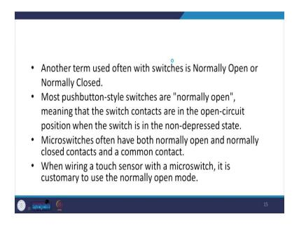
Now, another term which is often used in case of switches is normally open or normally closed. Most push button style switches are normally open it means that the switch contacts are in the open circuit position and the switch is in the non depressed state.
