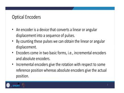
And by counting these pulses, we can obtain the amount of linear or angular displacement. And these optical encoders come in the two form, first is the incremental encoders and second is the absolute encoder.
