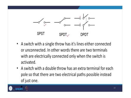
Here you can see that you have the single pole and the single throw, and here you have the single pole and double throw. There are two types of configurations that are possible in the double throw and here you have the double pole and double throw. With each the two configurations are possible.
