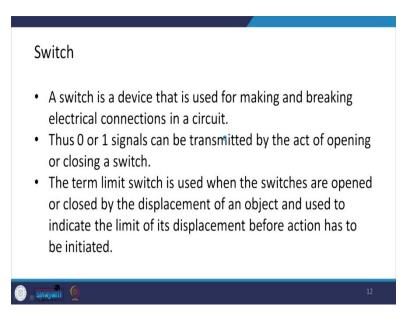
Another form of proximity sensors are switches and switches are in fact very cheap sensors. These switches are very similar to what we use in our house electrical connections. A switch is a device that is used for making and breaking the electrical connection in a circuit.
