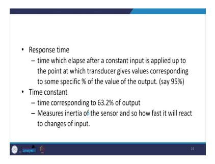
Then, there is term called response time, that is the time which elapse after a constant input is applied up to the point at which the transducers give values corresponding to some specified percentage of the value of the output, say 95 percent. So, your values are coming up to say 95 percentage of the specified value. So, what time it takes after giving the input that is what we call it as the response time.
