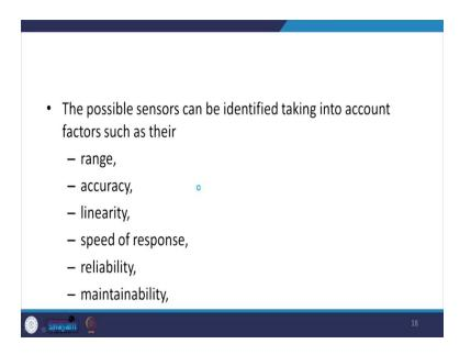
Then, the possible sensor can be identified taking into account factors such as, what is the range, what is the accuracy, how much up to, what value its linear behaviour is there, linearity, what is the speed of the response, how much reliable it is, how maintainable it is, what is the expected life.
