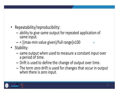
Then there is repeatability or reproducibility, as the name indicates we want to have our sensors repeatable. That is, they are able to give some output for repeated application of the same input. So, what we want that, if I am applying the same input number of times my sensor should be able to give the same output.
