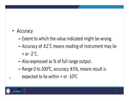
Then we often talk about the accuracy of the sensor, how accurate the sensors are? So, its definition is the extend to which the value indicated might be wrong. So, accuracy of  $\pm$  2-degree centigrade means reading of instrument may lie to '+' or - 2 degree centigrade. It is also expressed as percentage of full range output. Say if we are saying range is say 0 to 200 accuracies plus minus 5 percent means, result is expected to lie between plus or minus 10 degrees centigrade.
