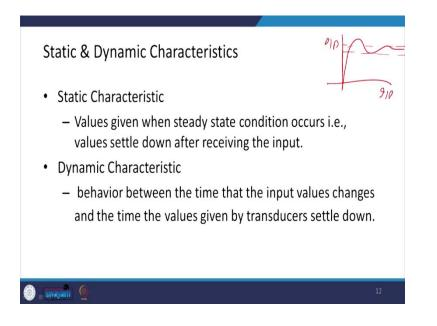
So, if I plot the input and output, we are interested in this zone that is the values gets settled basically. So, values given when steady state condition occurs that is value settle down after receiving the input.
