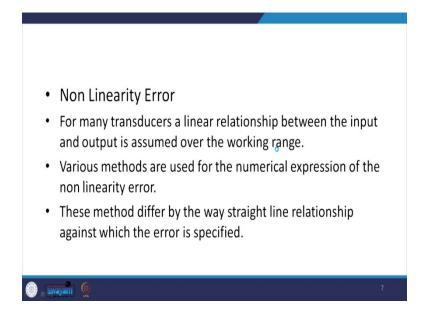
Then, we may have the non-linearity error. Non-linearity error is basically when we assume that the sensor behaviour is a linear one, but in the actual practice it may not be linear. In this type of situation the value predicted with the linear assumption that may not be correct. So, this is what is called as non-linearity error.
