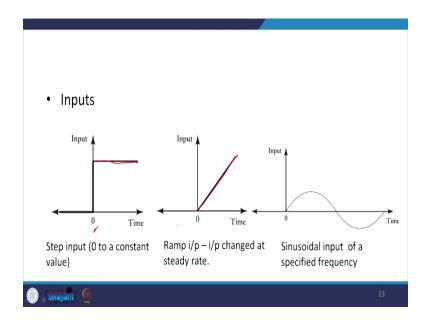
Now, the inputs which are used these could be the step input, that is the input varies from 0 to some constant value here. Then, the ramp input that is input changed at a steady rate as you can see here and which is given by a linear equation or we have the sinusoidal input. So, sinusoidal input of a specified frequency we may have like this.
