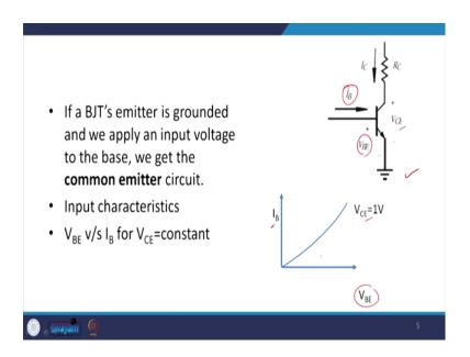
Now, if a BJT emitter is grounded and we apply an input voltage to the base, we call it as the common emitter circuit. So, this is the short notation for the common emitter connection. And, here input characteristic basically input is a  $V_{BE}$  that is  $V_{BE}$  versus  $I_B$ . So, if we plot  $V_{BE}$  versus  $I_B$  for a constant  $V_{CE}$  that is the voltage between collector and emitter. This is how we get the characteristic curve.
