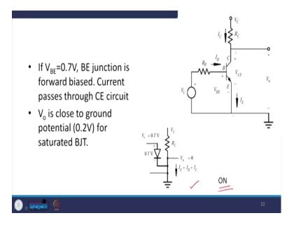
Now, if  $V_{BE}$  equals 0.7 volt, BE junction is forward bias and current passes through the collector that is CE circuit. And, in that case  $V_0$  is the output voltage is close to ground potential 0.2 volt for the saturated BJT. So, this is the condition which is shown for the saturation state and in this condition, we can see that the transistor is in the on condition. Because you have a lot of current flows through the  $R_c$ , that is  $I_c$  is large.
