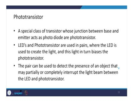
Then, we have another type of transistors called phototransistor. These are special class of transistors whose junction between base and emitter acts as a photodiode. And, these are what we call it as the phototransistors.
