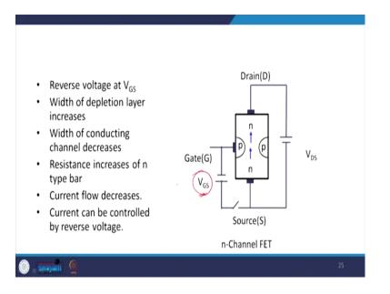
Now, if a reverse voltage  $V_{GS}$  is applied here, then what will happen is that the width of the depletion layer will increase. And, if width of depletion layer increases, width of conducting channel will decrease. And, because of this the resistance increases in the n type of bar and the current flow decreases. So, this is what we can see that, the current flow can be controlled with the help of this voltage  $V_{GS}$ .
