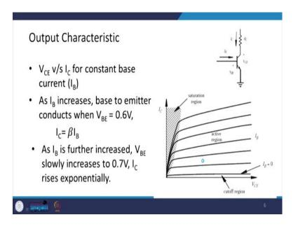
Now, let us look at the output characteristic. So, here for output characteristic, what we do is that we plot  $V_{CE}$  verses  $I_C$  for a constant base current value. So, we can see that as  $I_B$  increases, base to emitter conducts when  $V_{BE}$  value is around 6 volts. And, what we get  $I_C$  is equal to  $\beta$  times of the  $I_B$ , that is the current collector amplification.
