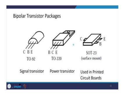
So, single transistor say T0-92 is this you have the collector port, base port, and emitter port. Similarly, the power transistors which are used in the power application is T0-220. These transistors could be of surface mount type, which could be used in the printed circuit board. So, they are just like say an example is SOT-23. So, here also we have collector base and emitter. And, this is how you get in the market.
