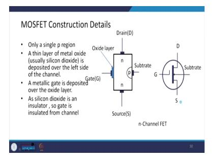
If we look at the MOSFET construction detail then here what we can find is that there is a source and a drain. And, in this case only one pn junction is there and a metal oxide layer usually silicon dioxide is put into it. At the top of it the gate is a metal is deposited over here.
