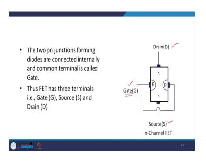
These two pn junctions forming diodes are connected internally and common terminal is called gate. So, FET has basically the three terminals, first is called Gate, second is called Source, and third is called Drain. These source and drains are interchangeable.
