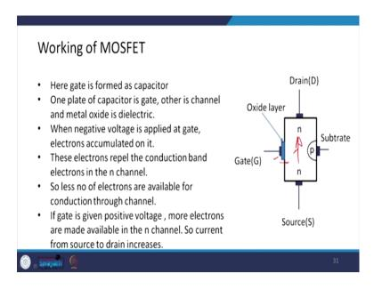
Now, let us see the working of the MOSFET. Here gate is formed as a capacitor. So, what happen basically, our gate is metallic and our channel is also metallic and there is an oxide layer in between. So, this oxide layer basically acts as a dielectric. This portion actually behaves as a capacitor. So, one plate of capacitor is gate other is channel and the metal oxide is dielectric.
