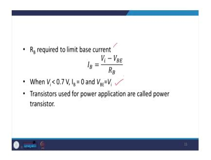
Now, what should the base resistor require to limit the base current. This we can find out by using the equation,
