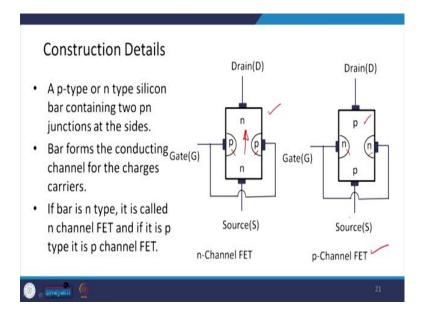
So, here a p-type or n type silicon bar contains two pn junctions at the sides. So, basically there is a bar, say this is a n type of bar and a p-type or n type silicon bar. So, this is your n type silicon bar, this is your p type silicon bar. And, this has got two pn junction at the side. So, one pn junction is here and another pn junction is here.
