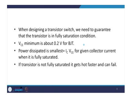
Now, when we are designing a transistor switch, we need to guarantee that the transistor is in fully saturation condition.  $V_{CE}$  minimum is around 0.2 volt for the BJT. And,
