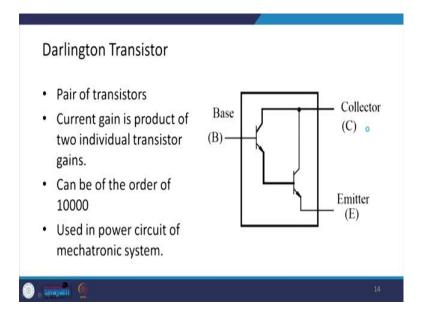
Now, there are type of transistors called Darlington transistors, which are often used in the mechatronic circuit. And, these are the pair of transistors basically the two power transistors, emitter is connected to the base of the second transistor. And, this way their collectors are connected together.
