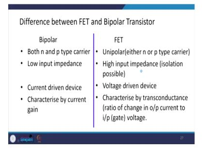
Now, coming to the difference between the FET and the bipolar transistor, the bipolar transistor current conduction is because of both n and p type carrier. Whereas, in case of field effect transistor current conduction is unipolar, that is either n type or the p type carrier will be conducting the current.
