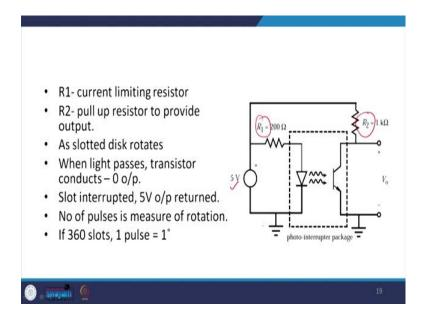
So, here is the circuit here, say this one is the current limiting resistor and this is the pull up resistor to provide the output. As slotted disk rotates, when light passes, transistor conducts and
