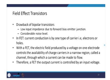
The bipolar transistor has certain drawbacks. These are that the low input admittance due to the forward bias emitter junction. We know that, the emitter base junction is the forward bias input side, and there is a considerable noise level.
