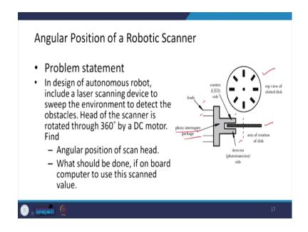
So, we can see that there is a photo interrupter package here, the leads are here for the connection purpose and there is a emitter that is LED side, and there is a detector here on phototransistor side. And, here this is a disk and axis of rotation of disk, if you see it from the top this is how it looks like.
