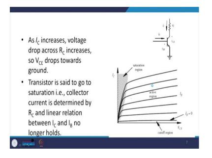
So, what happens basically as  $I_C$  increases there is lot of voltage drop across  $R_C$ . So, the  $V_{CE}$  drops towards ground its not 0, but it is very near to 0. And, the transistor is said to go saturation that is the collector current is determined by  $R_C$ . And, the linear relation between  $I_C$  and  $I_B$  no longer holds, this is what happens in the saturation region.
