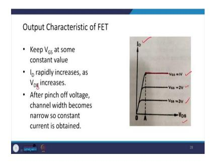
If we look at the characteristic of field effect transistor, then we can see that, if we keep  $V_{GS}$  that is the voltage between the gate and the source is at some constant value.  $I_D$  rapidly increases as  $V_{DS}$  increases basically. After pinch off voltage the channel width becomes narrow, and we get the constant current. These figures are shown for the different values of voltage between the gate and the source.
