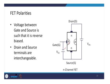
So, here the voltage between gate and source is such that it is reverse bias.
