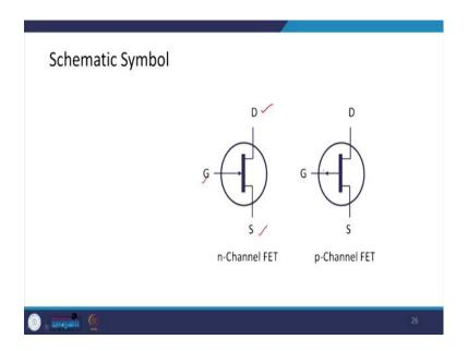
So, coming to the schematic for the FETs; this is for the n channel FET, we say source, gate, and the drain here. And, here in the n channel there is an arrow provided in this direction in case for the gate. And, for p channel again you have the three terminals, but here arrow is in the opposite direction. So, this is how they are symbolically represented.
