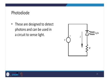
And similarly, there are photodiodes which works in the reverse wave, basically that is if light falls on them a current is produced. So, these are designed to detect the photons and can be used in a circuit to sense the light. So, photodiodes can basically work as a light sensor.
