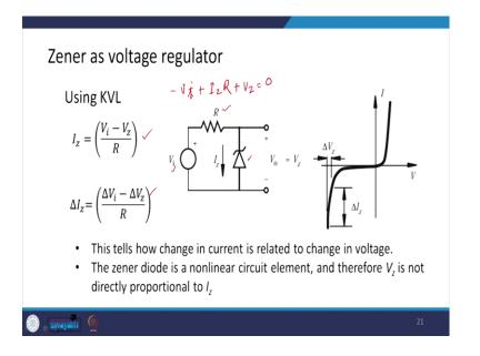
So, if we see zener as a voltage regulator, then the circuit with a voltage  $V_i$ , there is a resistor R and here is a zener diode and I am interested in using this zener diode as a voltage regulator, basically that is the one which gives me a constant voltage.
