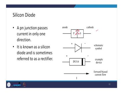
Now, here what we have seen that when the pn junction is forward biased, we get the current through it and when the it is reverse biased, there is no current; so, basically it passes current only in one direction that is the case when it is forward bias. So, silicon diode is that is why sometimes it referred as rectifier because it passes current only in one direction.
