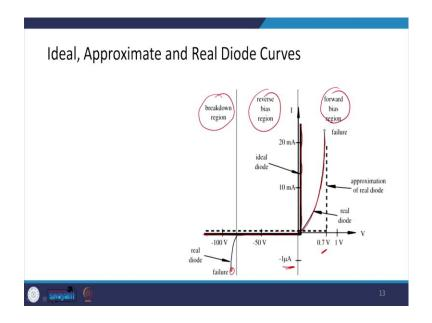
Now, I just discussed in the previous slide that there is a current flow if it is forward bias and there is no current flow if it is reverse bias. So, if we plot the voltage and current characteristic curve for the diode, then you can see that this is how it looks like.
