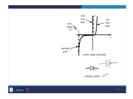
So, here we can see the schematic symbol of the zener diode, here you can see the difference whereas, for the normal diode, the symbol is this one. But in case of zener one, we have a different symbol and this is the V-I characteristic of it and here we are interested the zener being reverse bias. Here you can see that the voltage where we get current is called a zener voltage and this is the operating point around which we want to operate this.
