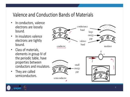
So, let us look at here some of the figures. Say for conductor, we can see that we have a valence band and we have a conduction band. In the conduction band, we have much number of free electrons are there and the segregation between the conduction band and the valence band or that is the energy gap which we call the forbidden energy gap. This forbidden band is very small or insignificant.
