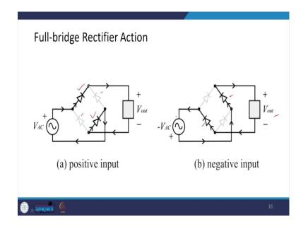
Now, how does this work basically? It is simple. So, if there is a positive input basically, so this is positive side; So, what happens? Positive side being connected to the positive side, so this is being forward bias. So, your current will be passing from here and similarly, this is positive side connected to the positive side so, forward bias.
