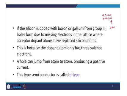
Now, if the silicon is doped with boron or gallium say from the group III, then holes form due to the missing electrons in the lattice where acceptor dopants atoms have replaced the silicon atom. Now, this is because the dopant atom only has got the three valence electrons.
