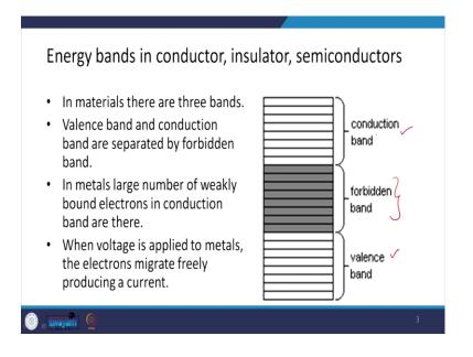
So, first of all, let us begin with the concept of energy bands in conductor, insulator and semiconductors. So, we can see that in any material essentially there are three bands; one is the conduction band and then we have the valence band and these two bands are separated by the forbidden band. It is the conduction band which is responsible for the conduction of the current basically.
