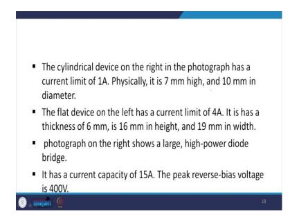
The cylindrical device on the right in the photograph as a current limit of 1 ampere. Physical, it is 7 millimeter high and 10 millimeter in diameter. The flat device on the left has a current limit of 4 ampere. It is it has a thickness of 6 millimeter and 16 millimeter height and 19 mm width and on the right there is a large high-power diode bridge which has current capacity of 15 ampere and peak reverse-bias voltage of 400 volts. So, these are the commercially available.
