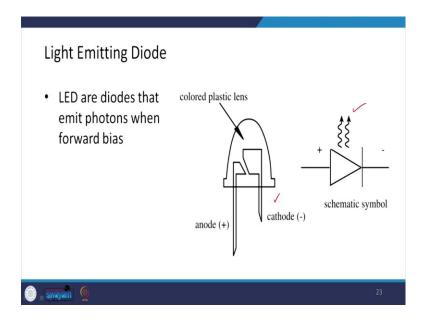
Then, there are a light emitting diodes basically these are the diode that emits photons when forward bias. So, this is the schematic representation for LED. So, photons being emitted when this is forward bias.
