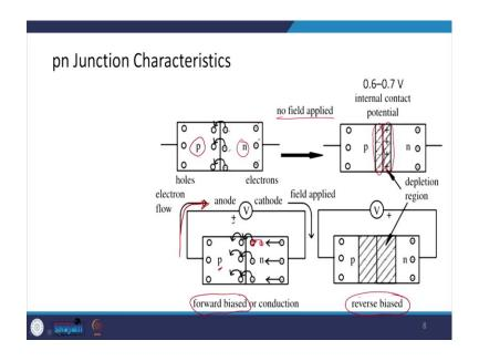
So, let us look at the pn junction characteristic, pn junction means what we are doing essentially is that a p-type semiconductor and a n-type semiconductor we are putting together. So, we have the p-type semiconductor, we have the n-type semiconductor. In n-type semiconductor, we have free electrons which are readily available to move, whereas in p-type semiconductor, we have the holes which are readily available to move.
