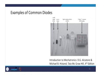
This figure shows basically some of the commercially available common diode. So, you can see small signal diode, power diodes are there, then LEDs or Light Emitting Diodes are there and 2-digits or 7-segment LED displays are there. So, you can see that there are 7-segments here 1, 2, 3, 4, 5, 6 and 7. So, these are what we call 2-digit 7-segment display because we can display the 2-digits with the help of 7-segment.
