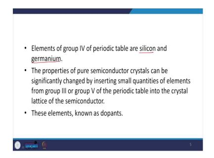
So, what happens if we look at the elements in group IV of the periodic table? Say we have silicon and germanium and the properties of pure semiconductor crystal can be significantly changed by inserting a small quantities of elements from either the higher group or say group V or the lower group say group III of the periodic table into the crystal lattice of the semiconductor. And this process is what we call it as the doping and these elements are basically called the dopants.
