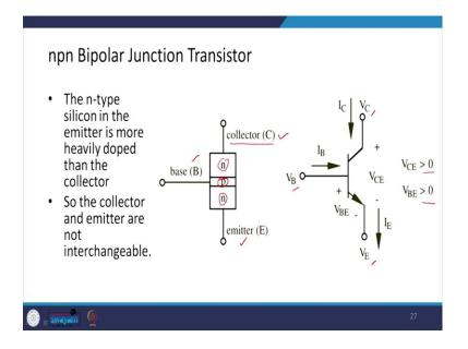
So, this figure you can see that it is a npn transistor basically. So, It is the p-type silicon, we have n-type silicon and n type silicon there. So, the one n terminal is connected here which is called collector, one center one is called base and here this is called emitter.
