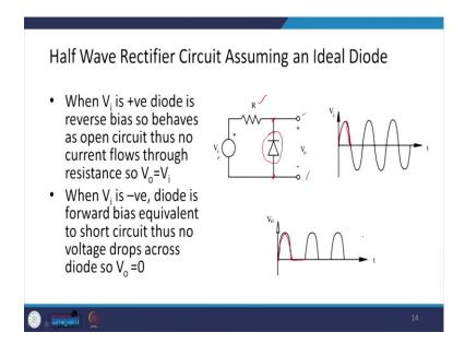
Now, this characteristic of the diode that it allows current only in one direction can be used for the rectification purpose. So, here, suppose I have got a voltage source  $V_i$  and this voltage is a varying say and let there is a circuit where we have a resistor and I am a putting diode over here and from this diode, I am typing the output voltage.
