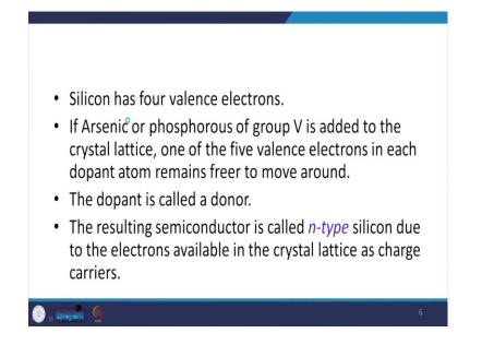
So, as I was telling you the silicon has got four valence electrons. So, if arsenic or phosphorus of say group V is added into the crystal lattice, then what happens? One of the five valence electron, we know eight electrons are required for the to get it as a saturated state.
