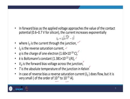
So, in forward bias as the applied voltage approaches the value of the contact potential say 0.6 to 0.7 volt for silicon, the current increases exponentially and this current is given by,
