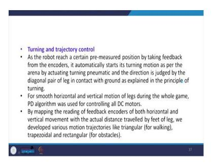
Then the turning and the trajectory control. As the robot reaches a certain pre-measured position by taking feedback from the encoder, it automatically starts its turning motion as per the arena by actuating the turning pneumatic and direction is just by the diagonal pair
