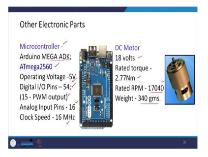
Other electronics parts used the microcontroller, Arduino MEGA ADK and ATmega2560 were used, and they have the operating voltage 5-volt, digital input-output pins 54, 15 PWM output is there, analog input pins are 16, and the clock speed is 16 MHz. Then, the DC motor is 18-volt, rated torque 2.77 Nm, rated RPM 17040, and weight approximately 340 grams.
