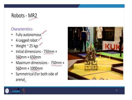
In the last lecture, I have talked about the Messenger Robot 1. In this lecture, I am going to focus on the technology development for the Messenger Robot 2. As we can see, these
