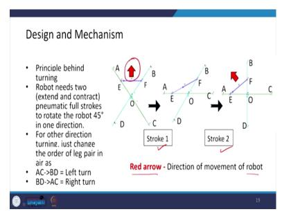
So, here the principle behind turning is that the robot needs two extend and contract full pneumatic strokes to rotate the robot  $45^{\circ}$  in one direction and for the other turning, the for the other direction turning, just change the order of the leg pair.
