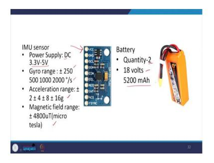
The IMU sensor which has been used is shown over here. These are the ratings for that power supply DC 3.3-volt to 5-volt, Gyro range plus  $\pm 250$  these are available so many degrees per second, acceleration ranges these are available, magnetic field range this much is available and the battery used, there was 2 number of such batteries of 18-volt and 5200 mAh current capacity.
