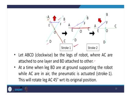
Here, ABCD is the leg of the robot, and where AC you can see is attached to the one layer and BD is attached to the other layer. Now, at a time when the leg BD is at the ground supporting the robot while AC is on the air, the pneumatic is attached, pneumatic has actuated the stroke 1, and this will rotate the leg AC by  $45^{\circ}$ , as you can see over here, which is like this and with this one actuation, this will be turning by  $45^{\circ}$  as over here.
