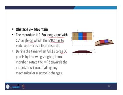
Now, let us look at the last obstacle that is not an obstacle rather a different type of terrine that is the mountain. The mountain is a 1.7-meter-long slope with a 15<sup>0</sup> angle on which the Messenger Robot has to make a climb as a final obstacle. During the time when Messenger Robot 1 scores 50 points by throwing shaghai, team members, rotate the MR2 towards the mountain without making any mechanical or electronic changes.
