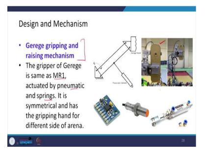
Now, let us look at the Gerege gripping and the raising mechanism. The gripper of the gerege is the same as the Messenger Robot 1, actuated by pneumatic and the spring. It is symmetrical and has the gripping hand for a different side of the arena. So, this is how you can see that this gerege has been gripped over here.
