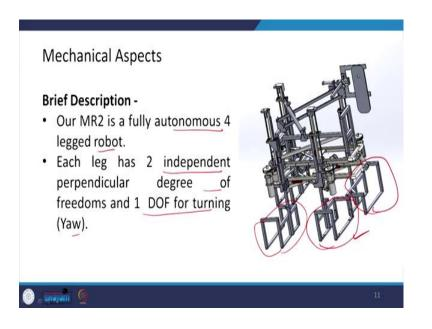
The mechanical aspect is a brief description of the robot developed by the IIT Roorkee team is that it is a fully autonomous 4-legged robot, and each leg has two independent perpendicular degrees of freedom and 1 degree of freedom for turning that is for the yaw motion, and this is the solid model of the robot which has been developed and here are the four legs so, this is 1, this is another one 2, this is three and the fourth one you have there in the background, in the backside.
