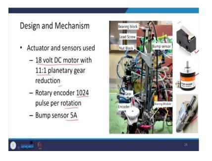
Actuators and sensors used are you can see the 18-volt DC motor with 11:1 planetary gear reduction. Rotary encoder 1024 pulse per rotation and bump sensor. So, here you can see this is the bump sensor, rotary encoder, and this is motor with the planetary gear reduction.
