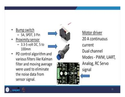
Then, the bump switch 5 ampere, single pole double throw, 3 pins. Proximity sensor, the 3.3 to 5-volt DC, 5 to 100 mm. Then, the motor driver 20 ampere continuous current dual-
