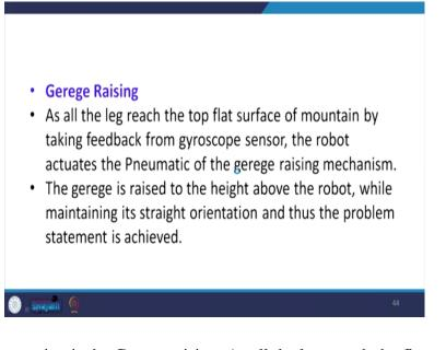
Next, the last operation is the Gerege raising. As all the legs reach the flat top surface of the mountain by taking feedback from the gyroscope sensor, the robot actuates the pneumatic of the gerege raising mechanism. The gerege is raised to the height above the robot while maintaining its straight orientation, and thus the problem statement is achieved.
