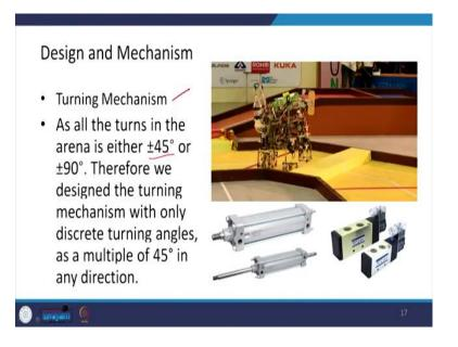
Then there is a turning mechanism for the robot to turn. So, all the turns in the arena are either  $\pm 45^{\circ}$  or  $\pm 90^{\circ}$ . Therefore, the IIT Roorkee team designed the turning mechanism with only discrete turning angles as a multiple of  $45^{\circ}$  in any direction.
