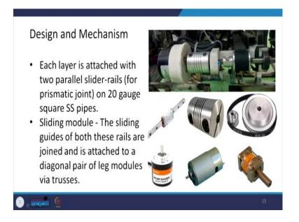
Then, each layer is attached with two parallel slide rails, as I said for prismatic joint on a 20-gauge square stainless steel plate.
