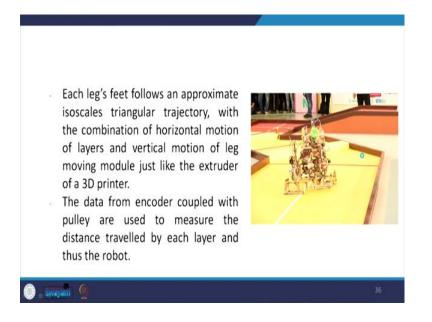
Now, each leg's feet follow an approximate isosceles triangular trajectory with the combination of horizontal motion of the layer and a vertical motion of the leg moving module, just like the extruder of a 3D printer. Now, the data from the encoder coupled with the pulley are used to measure the distance traveled by each layer and thus the robot.
