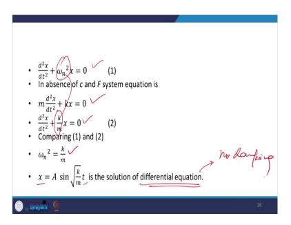
Now, if I compare this equation with the equation without damping, that is this one, then you can see that the,  $\omega_n^2 = \frac{k}{m}$ . So, I can write the solution as,
