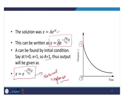
Now, if I substitute the value of *s*, this is the solution of the equation that I get. Here there is an initial *A* constant that can be evaluated by the initial condition. So, suppose at time t = 0 and put x = 1, so I will get A = 1 from here. So, this is the solution for the expression. So, this is what I said as the natural response. So, this is the natural response for the first-order system.
