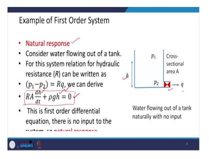
So, as I explained to you in the last lecture, suppose there is a tank, and there is a waterfilled up to a height h, and pressure at the top and bottom are  $p_1$  and  $p_2$  respectively and there is a wall through which the discharge takes place, and as  $p_2$  is the pressure hereafter the wall. So, we can write the expression for this as we have derived in the previous lecture. We can write the expression for flow through the wall, and the equation will be,
