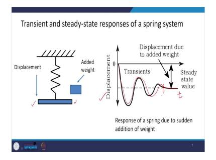
The example of transient and steady-state response, we can just consider a spring, and there is a hanger at the end of the spring, and if I add a certain weight to that hanger, then the spring will be getting displaced. So, this is how the displacement of the spring of if I plot with time, so this is how it is going to be. So, this is our transient response, and this part is the steady-state response. So, this is what I mean by the transient and steady-state response.
