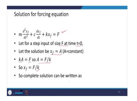
Now, the solution for the forcing equation if you look at this one. So, as we have seen for a step of size F at time t = 0, we can take the solution  $x_f = A$ . So, kA = F, so the A = F/k, and  $x_f = \frac{F}{k}$ .
