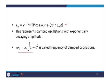
So, this is the natural response, and this one is called the damped frequency of oscillation, as I have explained to you.
