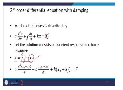
Now, what if there is damping? So, if damping is present, then this term is not going to be equal to 0, and we have the excitation force also F being over here. So, again here, I can take the solution to be composed of two forms is the natural response and the force response, and as we have done earlier, we can substitute this solution in this expression, and we can segregate the two parts over here.
