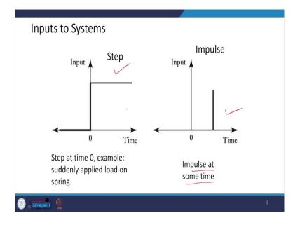
Now, the various input types of input can be used to excite the system. So, it could be a step input, or it could be impulse input, or it could be a ramp input, or the input could be a sinusoidal input.
