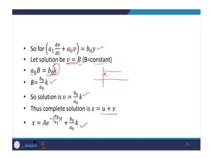
As I said, I can assume some solution for that v = B, which is a constant. If I substitute it over here, this term will become 0 because I am taking b as a constant. So, from here, I get the value of B. So, I get the solution. So, I can write the complete solution like this. This is the case for the solution of a first-order differential equation with a forcing function. (Refer Slide Time: 10:54)
