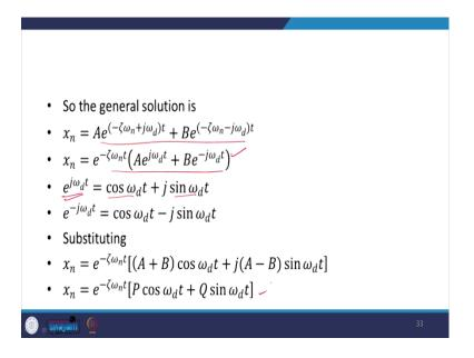
If I just substitute, I can further simplify this solution by representing the exponential function as cosine and sin functions. And this is going to be my natural response in that particular case.
