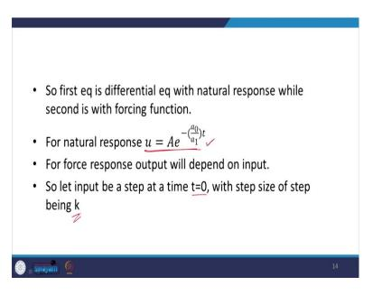
So, now let us try to find out the solution for the first equation that is with corresponds to 0 at the right-hand side over here. So, again it's the natural response. So, its solution is going to be this one. And for the force response, we can assume a step input, at t, is equal to 0 with a step size of k. If I do that, this is what is my equation.
