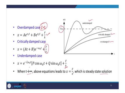
So, my complete solution I can write for all the 3 cases that are for  $\zeta > 1$ . I edit up here overdamped case, for the critically damped case, I edit up here, and for the underdamped case, I edit it over here.
