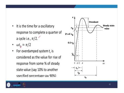
And it is the time for oscillatory response to complete a quarter of a cycle. So, this  $\omega t_r = \frac{\pi}{2}$ . So, this way we can find out the rise time. And for overtime system  $t_r$  is considered as the value for the rise of response from some percentage of the steady-state value, so 10 percent to another specified percentage 90 percent.
