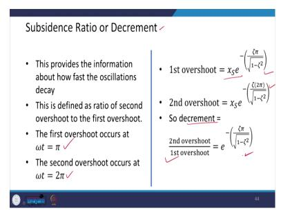
Then, the subsidence ratio or the decrement is again another major performance parameter. This provides information about how fast the oscillations are decaying, and it is defined as the ratio of the second overshoot to the first overshoot. So, the first overshoot occurs at  $\omega t = \pi$ , the second overshoot will be occurring at omega t is equal to  $\omega t = 2\pi$ .
