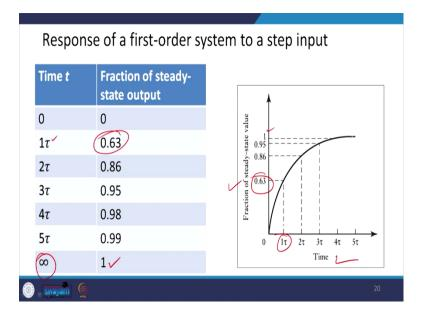
So,  $\tau=1$  or  $1\tau$ , this is 0.63. So, the fraction of steady-state value if I plot over time, so this is 0.63 at  $1\tau$ , and this way I can have the response, so you can see that at time infinity I get the steady-state value that is 1 over here.
