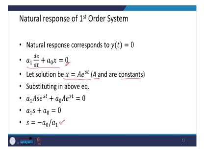
Now, if I talk about the natural response of the first-order system so, make the forcing function 0 here if I want to have the natural response. As it is a first-order differential equation, so its solution could be of form $x = Ae^{st}$ , where A and s are constants. And this if we substitute it over here then we can get the value of s as this one.
