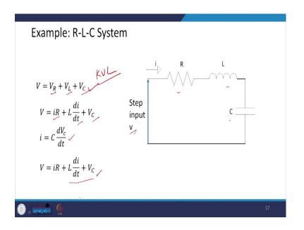
Another example, as I was telling you in the electrical system, it is a simple RLC circuit which is an example of the second-order system. We can, for a given step input I can write the Kirchhoff's Voltage Law, which is a KVL, and I can write this voltage across resistor, inductor, capacitor, and iR, Ldi/dt and  $V_c$  respectively. I can write it like this. So, this way, I can write an expression like this one.
