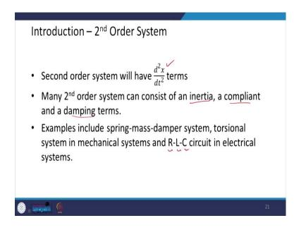
Next, let us talk about the second-order system. So, the second-order system, as we have seen that they have  $\frac{d^2x}{dt^2}$ . And the second-order system can consist of inertia, compliance, and damping for a mechanical system, and we have also seen on several occasions during this course the electrical system can have the resistor, inductor, as well as capacitor. They also represent the second-order system.
