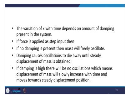
So, the variation of x with time depends on the amount of damping present in the system, and the force is applied as a step input, then. If there is no damping present in the system,
