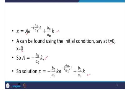
So, I can get the value of A by substituting that t = 0, x = 0. So, if I put it over here, I can get the value of a like this one. I can substitute it over here.
