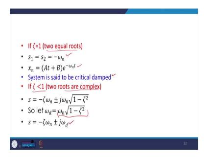
And if the  $\zeta = 1$ , this is going to be the solution, these are going to be the roots both equal, and this is going to be the solution, and the system is said to be critically damped. And if  $\zeta < 1$ , then the two roots that are complex are going to be there. We define this as the damped frequency, and the two roots can be represented like this. So, this is going to be the general solution.
