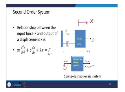
So, let us take the second-order system, a simple spring-mass damper system over here. So, this spring mass damper system is excited by an external force F. So, in this case, my input is F, and the output is this displacement x over here. So, I can write the equation of motion for this system by drawing the free body diagram, and it is this,
