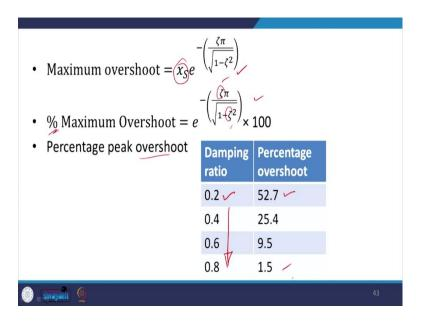
I am not working on the derivations over here. You can refer to the reference books which I will be telling you towards the end of this lecture. So, the percentage of the peak overshoot is going to be as you can function of the damping ratio over here. So, for the damping ratio, 0.2 overshoot is 52.7, and so on. So, as you can see, as we are increasing the damping ratio, the overshoot is decreasing. So, that is one of the observations which I wanted you to observe.
