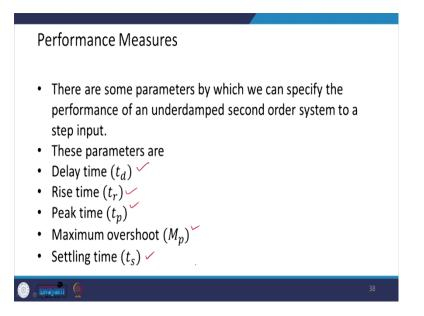
Then, there are various performance measures parameters, and these parameters are how the system is responding. Those parameters can be measured with the help of delay time, rise time, peak time, maximum overshoot, and settling time. So, with the help of these parameters, we can measure the performance of the dynamic system.
