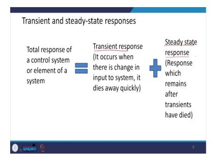
Now, the total response of any system is consists of the transient response as well as the steady-state response. Transient response is the one in which the change occurs when there is a change in the input to the system, and it dies away quickly. And the steady-state response remains, that is, the response that remains after the transients have died out.
