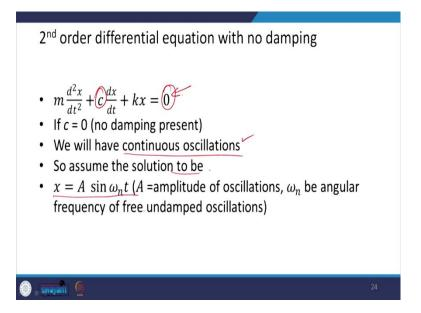
So, if there is no damping and there is no input excitation, I take here 0, and I have my input force 0, and I can take this c = 0. So, we will have because damping is not there, so we will have the continuous oscillations, and we can assume the solution of this form,
