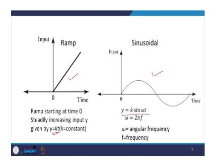
So, ramp input is defined as y = kt, sinusoidal we can define  $asy = ksin(\omega t)$ , and similarly, this impulse at some time and step has a certain value, at time t greater than 0. So, this way, these are the various types of inputs.
