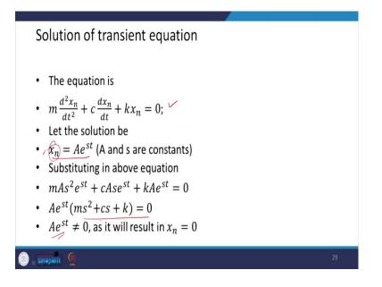
So, if we look at the solution for the transient equation that is for the natural response, so here I have I can take,  $x_n = Ae^{st}$  as the solution, and if I substitute it back over here. So I get this one, and this cannot be equal to 0 because if I make it is equal to 0, this itself will become 0, so I make the other equal to 0. So, this is my auxiliary equation. So, from here, I can get the value of s. It is a quadratic equation. So, its solution is going to be this form.
