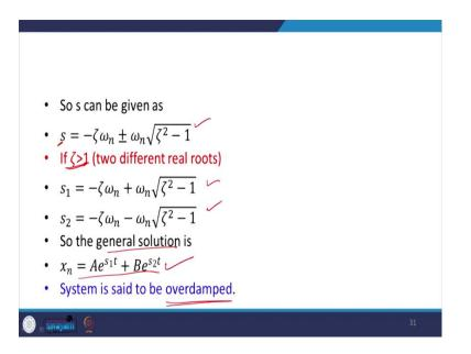
Now, here there are 3 cases, we are going to have this if  $\zeta$  is going to be more than 1, then these are the two solutions which I am going to get  $s_1$  and  $s_2$ , so the general solution is going to be this one. And we see that the system is overdamped.
