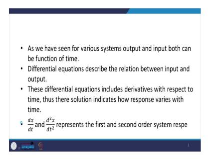
Various system output and input can be both a function of time, and we have seen that the differential equations are used to depict the relationship between the input and output, whether it is a first-order system or it is a second-order system. So, we see that  $\frac{dx}{dt}$  represents the first-order system and  $\frac{d^2x}{dt^2}$  represents the second-order system. Now, let us see the example of a first-order system.
