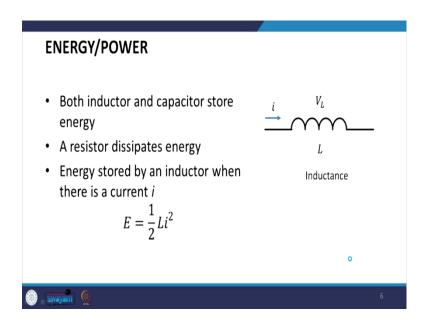
Now, what about energy and power? So, both the inductor and capacitor store energy, and a resistor dissipates energy. So, energy is stored by an inductor when there is a current *I*,
