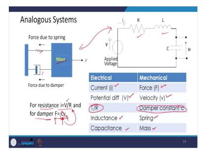
So, this way, using KCL and KVL, we can write the equation of the system. So, you see often there is an analogy which is made between the electrical system and a mechanical system. So, we have seen the mechanical system in the previous lecture, so where you have a mass, you have a spring, and you have a damper over here, and its analogous electrical system is an RLC circuit consisting of a resistor, inductor, and the capacitor.
