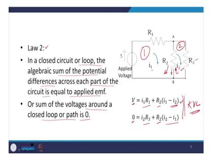
Then, there is the 2nd law by Kirchhoff, and it states that in a closed circuit or a loop, the algebraic sum of potential difference across each part of the circuit is equal to the applied emf or what we can that some of the voltages across a closed-loop or path is going to be 0. So, this law can be explained with the help of this very example over here.
