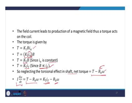
So, the field current leads to the production of a magnetic field. Thus, a torque at on the coil and this torque is given by,
