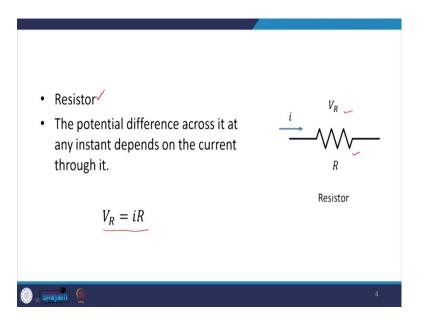
The next building block is the resistor which comes from the definition of the ohm, the definition for the resistor given by ohm's law. So, here the voltage drop across the ends of the resistor,
