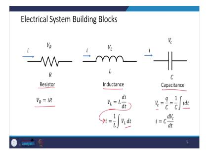
So, here are the three basic electrical system building blocks resistor, inductance, and capacitance.
