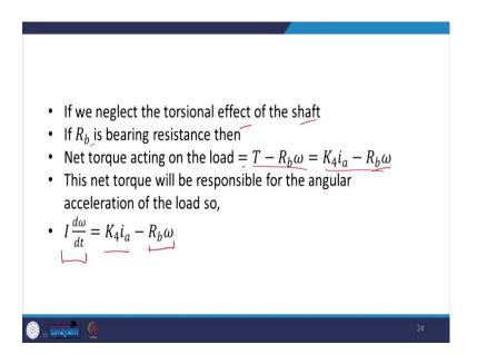
And if we neglect the torsional effect of the shaft and  $R_b$  is the bearing resistance, then net torque acting on the load is,
