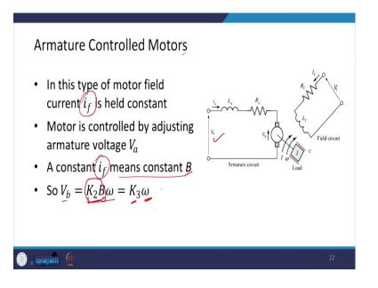
So, first, we will be looking at the armature control motor, and then, I will be talking about the field control motors. So, in the armature control motor, this type of motor field current is held constant because we are controlling it through the armature, and the motor is controlled by adjusting the armature voltage  $V_a$ , this one. So, a constant  $i_f$  means the constant B. As I said that we are taking  $i_f$  constant; so, a constant field current means a constant B. So,
