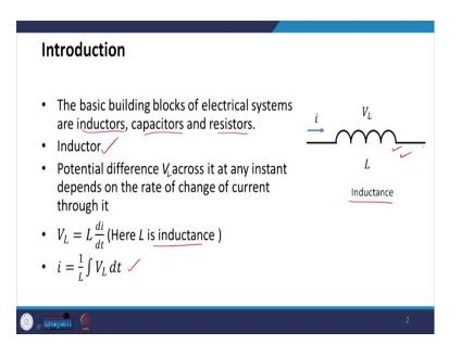
We see that this is the symbol for an inductor. So, the potential difference  $V_L$  across it at any instant depends on the rate of change of current through it. So,
