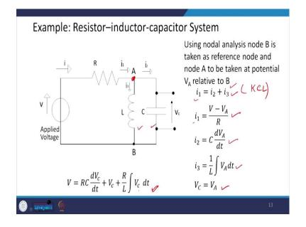
If we have a resistor inductor capacitor system here; in the previous case, all these R, L, and C, were in series and suppose here, they are in a parallel rest inductor and capacitor are in parallel, then, in this case, we can make a nodal analysis using Kirchhoff's current law. So, I will be getting this equation,
