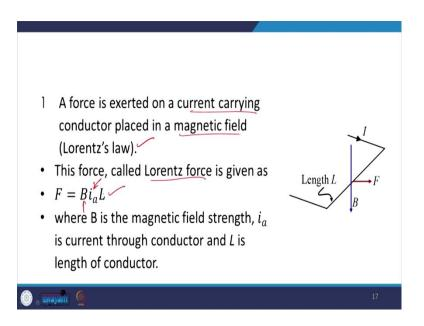
So, that is the basic principle. So, a force is exerted on the current-carrying conductor placed in the magnetic field. This is Lorentz law, and this force called Lorentz force is given by,
