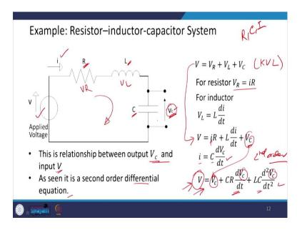
Now, next example, let us take where we have a combination of R C and I. So, I have got a resistor, I have got a capacitor, and I have got an inductor, and suppose my output, I am interested in seeing across the capacitor. So, this is my applied voltage or the voltage source, and here i is the current through the circuit.
