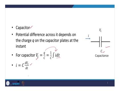
The next building block is the capacitor over here. So, see, there is a capacitor of capacitance C; the current through is i, and the  $V_C$  is the voltage across the plates over here. So, the potential difference across it depends on the charge on the capacitor plates at that instant. So, for here,
