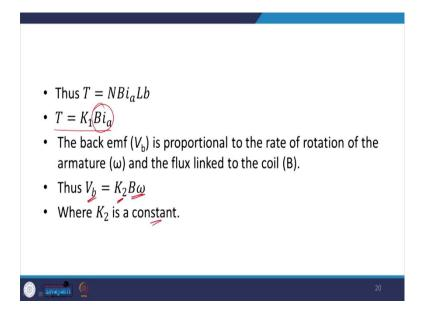
So, here suppose, if I am taking that B is also not constant, then we can take that the torque is proportional to B  $i_a$ . So, this is my equation,
