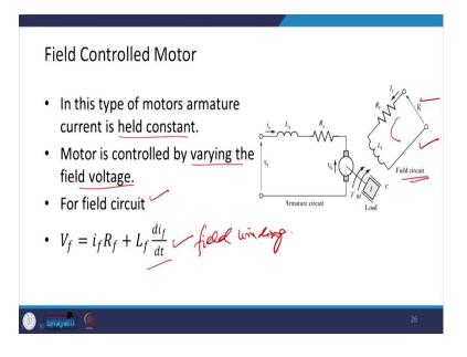
Next, let us take the field control motor. So, in the case of the field control motor, we are going to change the field over here. So, in this type of motor, armature current is held constant. So, the motor is controlled by varying the field voltage. So, for the field circuit here, I can write this equation that is,
