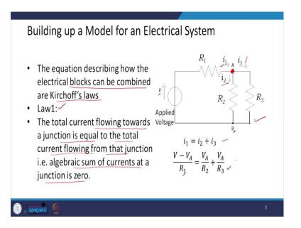
So, the equation describing how the electrical blocks can be combined is Kirchhoff's law, the combination of these blocks. So, the 1st law is the total current flowing towards a junction is equal to the total current flowing from that junction. So, the current in has to be equal to current out at a junction, or what we can is that the algebraic sum of current as it at a junction is 0.
