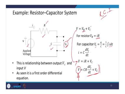
So, these are the building blocks for us if we want to model an electrical system. So, we have seen a resistor, we have seen a capacitor, we have seen an inductor. So, now, I am going to take the various combinations of these which exist in a circuit. So, here suppose I have a combination of resistor and capacitor.
