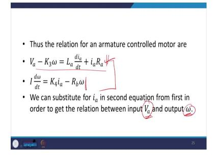
So, in the case of the armature control motor, we have got two relationships. This relationship which we have applied the Kirchhoff's voltage law for the armature and we have got and this relationship, we have applied for the load. So, this we have got.
