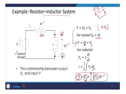
Next, let us take the example of the resistor and inductor. We have seen resistor, capacitor, and inductor. So, in the last slide, I have shown you the example of resistor and capacitor. Next, let us see an example of having the combination of resistor and inductor. So, you have a resistor, and you have an inductor over here. So, again my input is applied voltage V and output suppose I want to take across the two terminals of the inductor that is my output.
