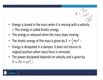
So, energy is dissipated in the damper. It does not return to the original position when the input force is removed. Why does it not return to its original position? Because it has dissipated the energy. And the power dissipated depends on the velocity, and this is given by this power is given by force into the velocity. And this force is a damping force.
