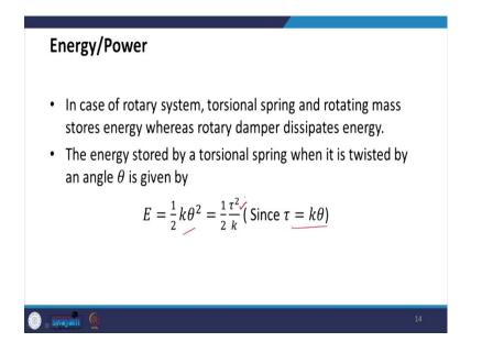
So, the energy is stored in torsional spring when it is twisted by an angle  $\theta$  is given by,
