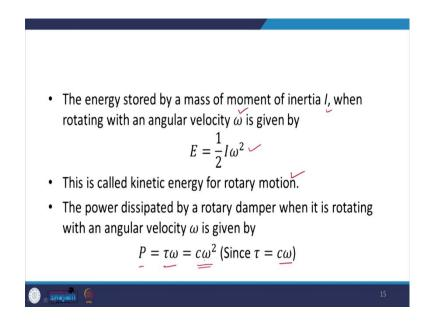
And the damper dissipates energy. So, the power dissipated by the rotary damper when it is rotating with angular velocity is given by,
