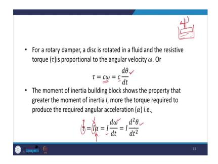
So, for a rotary damper, a disk rotates in a fluid, and the resistive torque here you have got the fluid, and the resistive torque is proportional to the angular velocity  $\omega$ .
