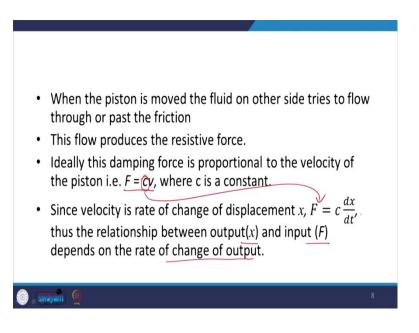
And ideally, the damping force is proportional to the velocity of the piston, and you have (F=cv) here, where c is a constant. And you see the velocity is what? Velocity is the rate of change of displacement. So, I can write this as,
