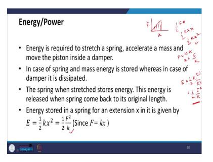
Now, as I said, for spring and mass, the energy is stored, whereas, in the case of a damper, it is then dissipated to the environment. And the spring, when you stress it stores energy, and this energy is released when spring comes back to the original length. And you know energy is stored in the spring is given by spring for a given extension, x is
