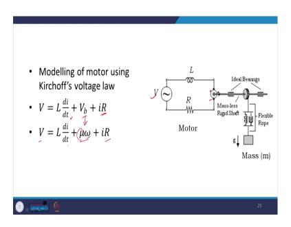
So, modeling the motor is pretty simple. We can use Kirchhoff's voltage law to model it. So, this V will be  $L\frac{di}{dt}$ . That is the voltage drop across the inductor plus the back emf, which will be generated at the motor plus the voltage drop at the resistor iR. So, this is,
