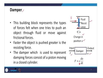
So, the damper has you can see that there is a cylinder and piston arrangement and there is a fluid inside of this. When this piston is moved, then this fluid is passed to allowed to pass through these constricted spaces, and this produces resistance. So, here because of the motion, there is a change in position x here.
