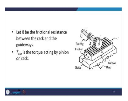
So, let R be the frictional resistance between the rack and the guideway. And  $T_{out}$  is the torque acting on the pinion torque acting by the pinion on the rack.
