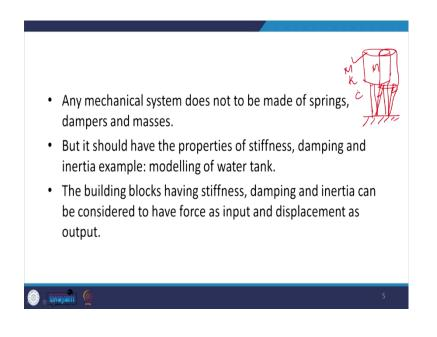
I mean by this that there may not be all these three elements present in that mechanical system to identify, as well as they should, but it should have the properties of stiffness, damping, and inertia. So, in a real system, you will not have these spring, mass, and damper systems, but whatever is present in the system that will have this type of property.
