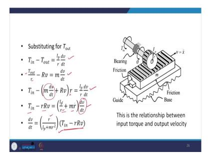
So, we had this equation, and we had this equation. The relation between input torque and output velocity is,
