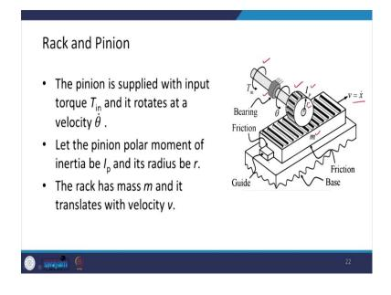
So, here we can see a schematic diagram. I have got a pinion with the moment of inertia,  $I_p$ , the radius is r a and torque  $T_{in}$  is input torque is applied over here. There is bearing friction. And I have got a rack which has got a mass *m*, it has got a velocity, and there is friction over here, and there is a guide.
