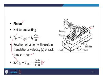
So, let us write the equation of motion first for the pinion,
