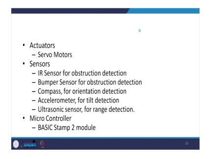
So, actuators here are servo motors which are being used and the sensors which are attached with this kit are IR sensor for obstruction detection that is infrared sensor, then we have the bumper sensor for obstruction detection. Basically, these bumper sensors are nothing but the just like switches basically so, they make on and off contact ok.
