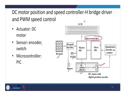
Next another example I wanted to tell you where the DC motor is being used as an actuator ok. So, here the DC motor position and speed controller that is through H-bridge driver and pulse width modulation speed control that is PWM control.
