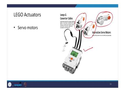
Coming to the actuators, so servo motors are there. So, here with the kit, the three servo motors are provided and these servo motors can be connected through the controller over here ah. So, these servo motor ensures that the robot moves smoothly and precisely.
