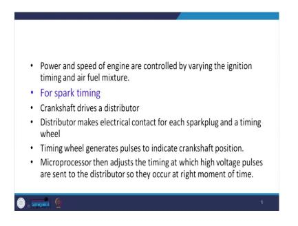
So, the power and speed of engine are controlled by varying the ignition timing and the air fuel mixture ok. So, what happens actually? For spark timing what is done is that crankshaft drives a distributor and distributor makes electrical contact for each spark plug and a timing wheel.
