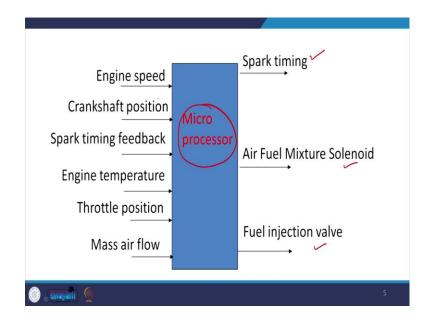
And with the help of mechatronics, what is done is that we try to control spark timing, we try to control air fuel mixture and we try to control the fuel injection ok. So, we have a actually microprocessor as you can see in the this block diagram, there are various input parameters over here. For example, we have engine speed, crankshaft position, spark timing feedback, then engine temperature is there, throttle position is there and mass of mass air flow is there ok.
