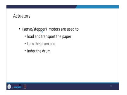
Coming to the actuators, there are servo motors and stepper motors which are used to load and transport the paper turn the drum and index the drum ok. So, these are the that is the three operations for which the actuators are used and we may have servos as well as the stepper motor for this purpose.
