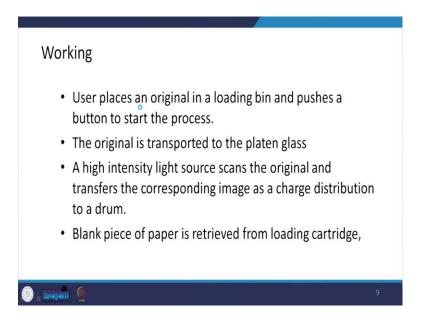
If we look at the working of the copy machine, here are the various steps first of all what one does is that is the user places an original which is to be copied in a loading bin and pushes button to start the process.
