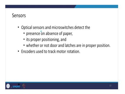
Now, what are the sensors in this? There are optical sensors and micro switches to detect the presence or absence of paper whether the paper is present or not, its proper positioning, so that you get the proper copy of it and whether or not door and latches are in proper position. So, for these optical sensors are used and the encoders are used to track motor rotation. So, these are the sensors which are used in this mechatronic system.
