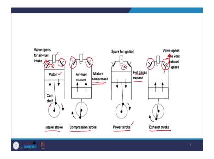
Here, in this figure, we can see the various four-strokes are mentioned intake stroke, compression stroke, power stroke and the exhaust stroke. So, we can see in this figure the
