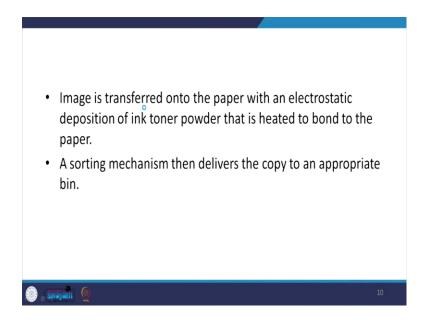
And then, the image is transferred into that blank paper with an electrostatic deposition of ink toner power powder that is heated to bond to the paper and then finally, a sorting mechanism delivers the copy to an appropriate bin. So, these are the steps in a copying machine.
