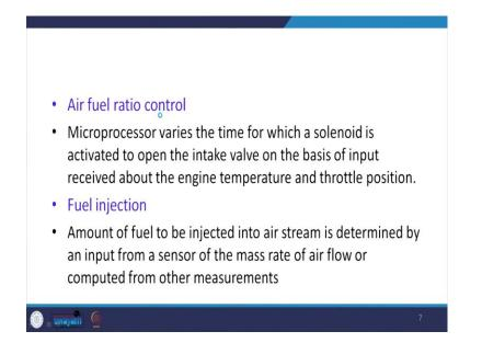
Similarly, for air fuel ratio control, what is the done is that microprocessor varies the time for which a solenoid is activated to open the intake valve on the basis of input received about the engine temperature and the throttle position. So, with engine temperature and throttle position as the input, microprocessor controls the opening of the solenoid valve ok. So, this is how it is done.
