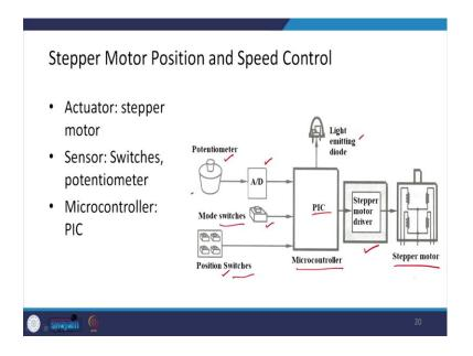
Similarly, we can look at stepper motor position and speed control ok. Now, if we look at this figure, here we see we have a say stepper motor, here there is a stepper motor driver and this driver is connected through a PIC microcontroller and then we have modes for input that is a potentiometer, then we have one analogue to digital converter is there, there are mode switches and there are position switches and you have the light emitting diode here just to see the working of it.
