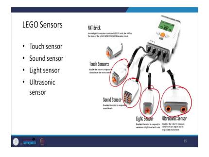
So, coming to what are the Lego sensors available in this so, there is a touch sensor, there is a sound sensor, there is a light sensor and the ultra ultrasonic sensor is there ok.
