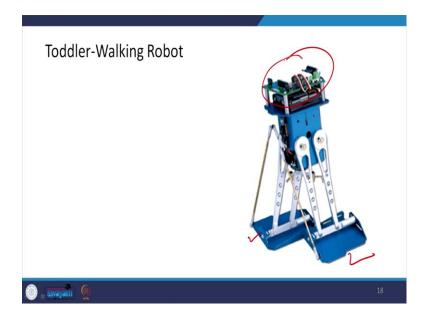
Next example is the toddler-walking robot which I want to talk to you. It is a basically a twolegged robot and again, there are various mechatronics components in it, there are sensors, there are actuators and there is a microcontroller as you can see here and there are sensors.
