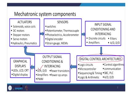
A digital to analog converter is used in the output signal conditioning and interfacing. So, as I have been talking to you that the signals which we get from the microprocessor are digital control architecture. These signals are digital in nature and these signals need to be converted into the analog signal if you want to send or if you want to send those signals to an actuator. Then we require the digital to analog converter.
