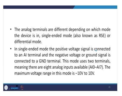
The analog terminals are different depending on which mode the device is in single-ended mode also known as RSE or different mode. In single-ended the positive voltage signal is
