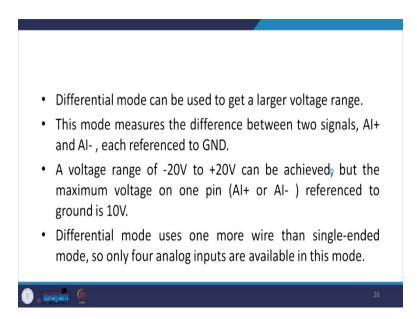
Differential mode can also be used to get larger voltage range and this mode measures the difference between the two signals. So, AI + and AI- each reference to the ground. A voltage ranges of -20 volt to 20 volts can be achieved, but the maximum voltage on one pin that is AI+ or AI- reference to the ground is 10 volts. Differential mode uses one more wire then single ended mode, so, only 4 analog inputs are available in this mode.
