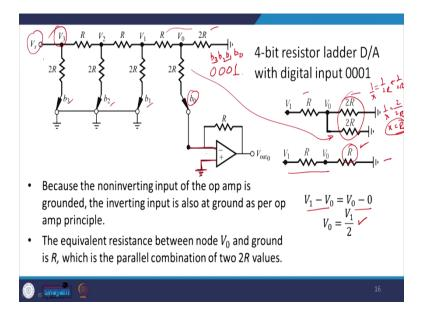
So, as we can see over here. So, this corresponds to 0001. So, here you can see that this one b 0 is connected to the op amp inverting terminal over here and b 1, b 2, b 3 these are
