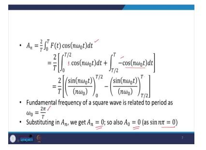
Now, this waveform if I want to represent mathematically that is the using the Fourier series, then we can evaluate the different components here. That is, we can evaluate  $C_0$ , we can evaluate  $A_n$  and we can evaluate  $B_n$ , then we can see that how we can represent this signal. So,
