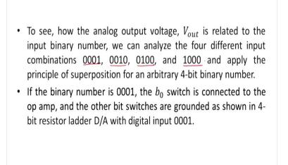
Now, to see how the analog output voltage  $V_{out}$  is related to the input binary number. We can analyze the four different input combinations 0001, 0010, 0100 and 1000 and apply the principle of superposition for any arbitrary 4-bit number, and let us start with the first one. If the binary number is 0001 the  $b_0$  switch is connected to the op-amp and the other bit switches are grounded.
