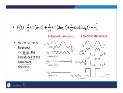
So, this is how F(t) is represented over here. So, this is the Fourier series representation of the square wave signal of the unit amplitude; so, now if you look at the individual harmonics and combined harmonics. So, this  $\omega_0$  frequency here we have the amplitude as  $4/\pi$ , this is the waveform, and  $3\omega_0$  as amplitude  $4/3\pi$ .
