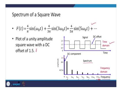
So, the spectrum of a square wave this is your F(t). So, plot of unity amplitude square wave or with a DC offset if this is 1.5 volt. Then in the time domain if I plot it, this is how the signal is going to lo like and its spectrum is something like this frequency.
