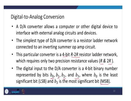
Now, let us talk about digital to analog conversion. The digital to analog converter allows a computer or other digital device to interface with external analog circuit and devices as I talk to you. These devices could be the actuator. The simplest type of digital to analog converter is a resistor ladder network connected to an inverter summing operational amplifier circuit. So, that I am going to discuss with you.
