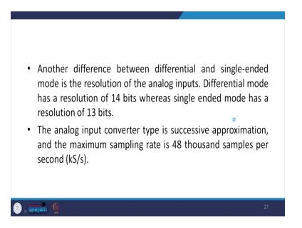
Another difference between differential and single ended mode is the resolution of the analog input differential mode has a resolution of 14 bit whereas, single ended mode has a resolution of 13 bit. The analog input converter type is a successive approximation which I have already discussed with you and the maximum sampling rate is 48 thousand samples per second.
