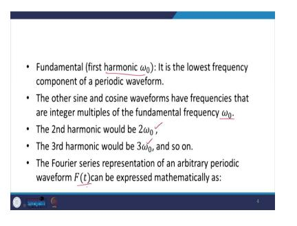
So, the fundamental or the first harmonic frequency  $\omega_0$  is defined as the lowest frequency component of a periodic waveform. The other sine and cosine waveforms have frequencies that are integral multiples of the fundamental frequency  $\omega_0$ . So, the 2nd harmonic would be represented as  $2\omega_0$ ; the 3rd harmonic will be represented at  $3\omega_0$  and so on. The Fourier series representation of an arbitrary periodic waveform F(t) can be expressed mathematically as this.
