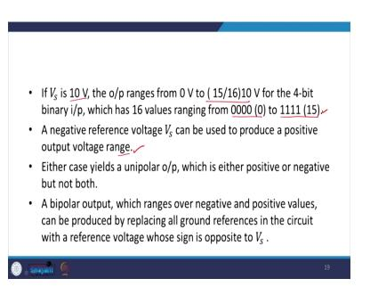
Now, if  $V_s$  is 10 volt the output ranges from 0 volt to (15/16)10 volt for the 4 bit binary input which has 16 values ranging from 0000 which is the 0th one to 1111 which is the 15th one. And, a negative reference voltage ( $V_s$ ) can be used to produce a positive output voltage range.
