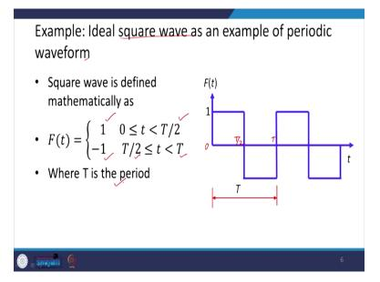
So, suppose we have a ideal square wave as an example of the periodic waveform. So, I have an ideal square wave whose magnitude is 1 between 0 to T/2, and between T/2 and T, it is -1, where T is the period. So, the square waveform is defined like this.
