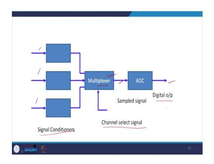
The scheme could be like, you have a signal conditioning conditioner unit. There are multiple signals like this. You pass it through a multiplexer over here. There is a channel to be selected. And, you have a sampled signal here and then it can be sent to analog to digital converter and you get the digital output from over here.
