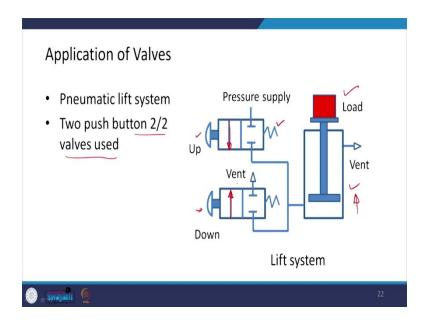
Then, there are these valves can have various applications such as a pneumatic lift system. And, in this pneumatic system, you could have a load here, and you could have a cylinder piston type of arrangement say over here, and we can use that two push 2 by 2 valve can be used.
