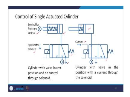
Control of single actuated cylinders; these are the two symbols that I am using the for pressure source and for the exhaust.
