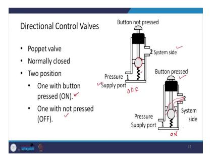
Now, poppet valves if we talk about poppet valves, they are normally closed. So, this is how the poppet valve configuration is so, you have this device here, there is a ball over here and you have a spring, this is the pressure supply port and this is the system side port. So, if the button is not pressed so, you can see that this is there in a closed position because this is spring. So, the spring keeps this valve closed position.
