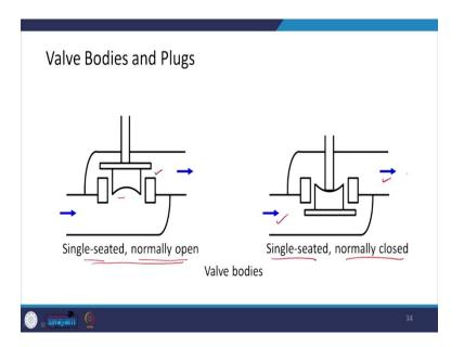
There are various types of valve bodies and plugs, this is a single-seated normally open. In this, there is only one seat and normally this is open condition. So, this is called singleseated normally open and this is single-seated and this is normally closed condition. So, in normal conditions liquid cannot flow from this side to this side.
