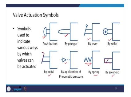
Now, there are various valve actuation symbols that are used. So, this is the symbol for the push button, this is the symbol for the plunger. So, here it looks like a button. So, if this symbol is there it means that the valve actuation is through the push button, this is valve actuation through the plunger, this is for using a lever, this is using a roller, this is by a pedal; a pedal shape is here.
