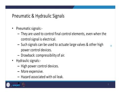
The pneumatic devices used air as the medium. So, they are used to control final elements even when the control signal is electrical.
