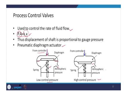
Next, let us lo at the process control valve. These are used to control the rate of fluid flow. And, in this case, what is what happens is there is a diaphragm as you can see over here, this side is connected to the controller. There is a spring over here, this is atmospheric pressure to this side and there is low control pressure is there.
