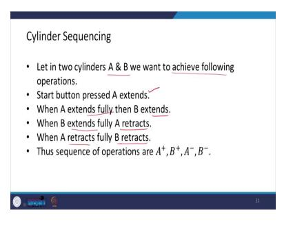
There could be a cylinder sequencing operation also. I am not going to talk much in detail, you can refer to mechatronics by Bolton if you are further interested in how the cylinder sequencing could be done.
