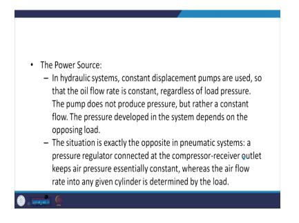
Coming to the power source in the hydraulic system, we use constant displacement. So, that the oil flow rate is constant regardless of the load pressure. The pump does not produce pressure, but rather a constant flow. The pressure developed in the system depends on the opposing load.
