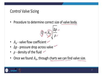
Then, we can also look at the control valve sizing. The procedure to determine the correct size of the valve body,
