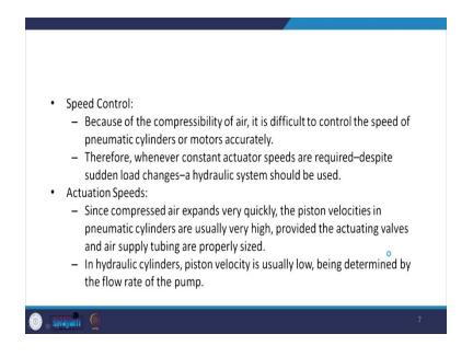
So, whenever constant actuator is speed is required, despite certain load changes we go for the hydraulic system, fine. What about actuation speed? Since compressed air expands very quickly, the piston velocities in the pneumatic cylinder are usually very high and they provide the actuating valves and air supply tubing are if they are properly sized and so, they do it quickly. Whereas in the case of hydraulic cylinder piston velocity is usually low being determined by the flow rate of the pump.
