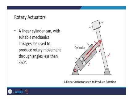
There are rotary actuators. They have a cylinder and piston arrangement. And this cylinder this your piston could be used to drive some lever over here. In this way, we are converting this piston motion into this thing rotary motion.
