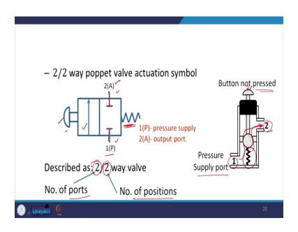
It is a pressure supply port and it has the here, port number 2 which is connected to the application side. And, you see that this valve has how many, it has how many ports? It has 2 ports. So, these are the 2 ports.
