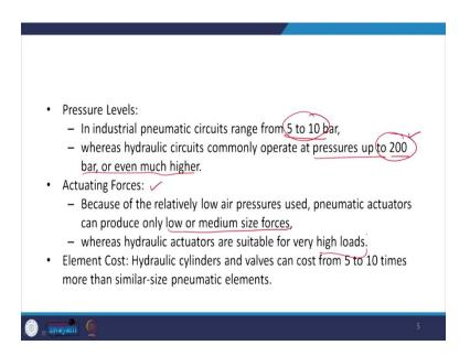
Let us see what are the differences between the two that are hydraulic and pneumatic systems. So, first of all, let us differentiate at the pressure level. In an industrial pneumatic
