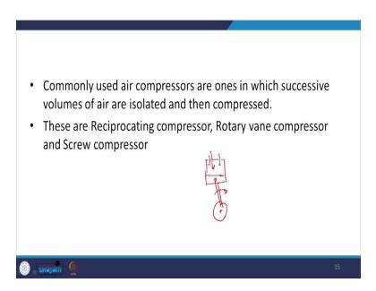
Commonly used air compressors are one in which successive volumes of air are isolated and then compressed. These are the reciprocating compressor, rotary vane compressor, and screw compressor.
