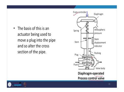
And, these types of devices that are the process control valve, could be used to operate certain valves such as diaphragm operated process control valves. Here, you can see that some fluid is going, and here is a valve, and this valve could be controlled with the help of this device from the controller.
