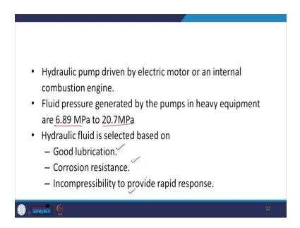
So, hydraulic pumps are driven by an electric motor or internal combustion engine that could be there. And, fluid pressure generated by the pump in heavy equipment is said from 6.89 mega Pascal to around 20.7 mega Pascal.
