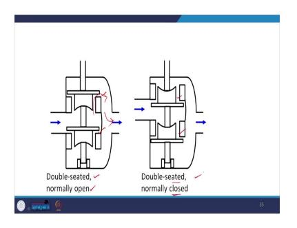
Then, we have double-seated, there are double seats one seat here, another seat here. So, this is called double seated and normally open. It is normally open so, the liquid can flow this way. And, this is the double-seated that is a seat here and here and this is the normally closed configuration.
