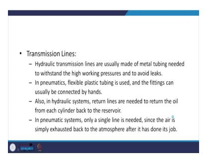
And you see in the hydraulic system the working fluid is costly. So, unlike the pneumatic system, where we can allow the air to escape to the atmosphere, in the hydraulic system we cannot allow the oil to escape into the atmosphere. So, we need the return line to return the oil from each cylinder back into the reservoir.
