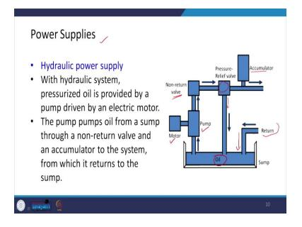
Let us look at it one by one. So, first of all, we will be looking at the hydraulic power supply. Now, in the hydraulic power supply as I said we are using oil. So, there is a sump where oil is there now, this oil is pumped with the help of a pump and this pump is actuated by a motor. Now, oil from the pump goes to a non-return valve. So, that oil does not come
