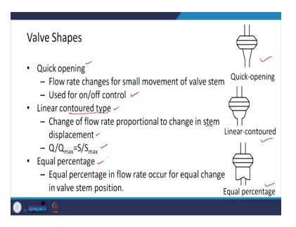
There are various shapes of the valve for quick opening, linear contoured, and equal percentage. These types of quick opening valve flow rate change for a small movement of the valve stem as the name indicates, they are quick reckoning and these are used for the on-off control. Then, in the linear contoured type, the change of flow rate is proportional to the change in a stem displacement.
