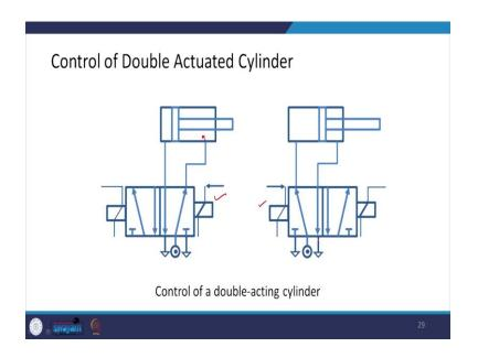
Then, we could have control for the double-acting cylinder also. So, in the case of a doubleacting cylinder, when this solenoid is acting, you have the flow from this one, and exhaust takes place from here alright. And, when this is solenoid is acting in that case you have flowed from this side and exhaust takes from this side.
