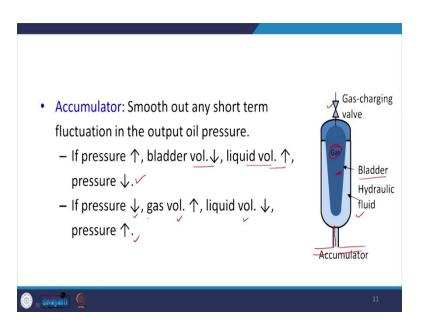
Now, what is this accumulator? So, this accumulator is a device to smooth out short-term fluctuation in the output oil pressure, and how this is done? So, this device has got a there is a bladder, on which gas is there. And, there is a gas charging valve through with this gas can be charged and there is a hydraulic fluid over here.
