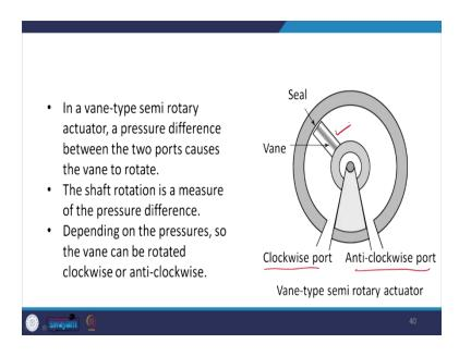
Then, we could have a various vane type semi-rotary actuator, a pressure difference between the two ports causes the vane to rotate and the shaft rotation is the measure of the pressure difference. And depending on the pressure, the vane can be rotated clockwise or anti-clockwise. So, essentially it has got a clockwise port and anti-clockwise port and there is a vane .
