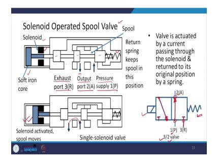
So, I have this spool valve this is the rod and these are the pistons and this is actuated by the solenoid over here. So, there is a soft iron core and you have a solenoid, I just said I will be talking about this solenoid in my electrical actuation devices lecture.
