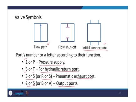
Now, in a circuit hydraulic circuit, there could be many types of valves being used. So, to represent the action, we use the valve symbols. And, these valve symbols say we in these valve symbols, we indicate the flow path like this and if the flow is shut off, then it is indicated like this. And, this configuration indicates the initial connections.
