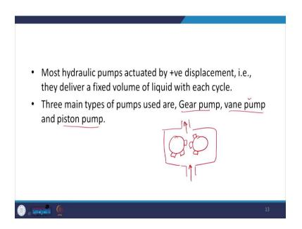
So, the two gears are there like this and these gears are in mesh. So, something like this they are there this device is there in a casing. And you have the input from here, and you have the output from here and it compresses and displaces the liquid. Similarly, the vane pump has got vanes, which displace the liquid and likewise with the piston pump.
