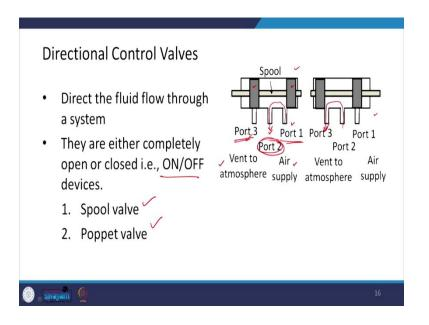
So, the same principle is used in your IC engines. Then, the other element is the directional control valves. So, as the name indicates they direct the fluid flow through a system, and they are either completely open or closed or what we call the ON-OFF devices. So, these are of two types the spool valve and the poppet valve.
