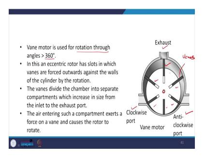
So, this is the vane type of rotary actuator. The vane motor is used for rotation if we are looking for rotation more than 360 degrees. And in this eccentric rotor has slots in which the vanes are forced, outward against the valve of the cylinder. So, here you can see that these are the vanes. And, these are forced across the valve of the cylinder.
