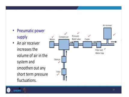
Now, let us lo at the pneumatic power supply. So, the pneumatic power supplies are something like this. So, you have to take in the air. So, there is a filter to remove the dirt
