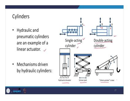
There are various mechanisms that could be driven by hydraulic cylinders. These cylinders could be either single-acting, or they could be double-acting.
