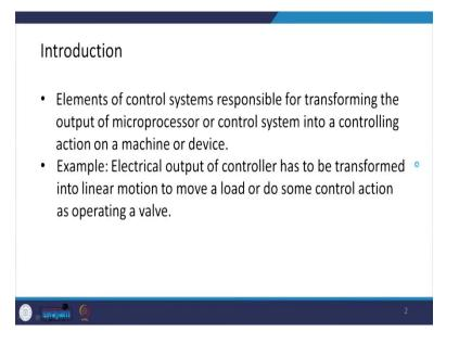
For example, I can take the electrical output of a controller has to be transformed into say linear motion to move a load, or to do some control action say operating of a certain valve of the hydraulic system or say some valve of the pneumatic system. So, this is where these
