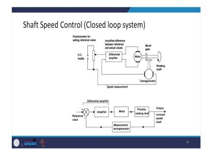
So, the example of this closed loop system is the shaft speed control, where we can see that, there is a motor here and we tap the output speed of the motor, so with the help of the shaft of the bevel gear in the bevel gear arrangement, a tachogenerator is driven basically.
