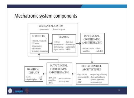
So, here basically we can see the mechanical systems, on mechanical systems basically we have the actuators and sensors; actuators could be say solenoid, voice coils, DC motors, stepper motor depending on what application you are interested stepper motor, servo motors,
