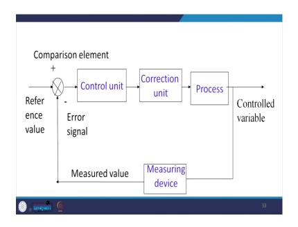
Now, here basically if we talk in general term; so we have a control unit, we have a correction unit, and we have a process. And the controlled variable of course, is taken from here through the measuring device and the measured value is given to the comparison element, where the error signal is found.
