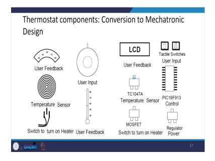
Now, if we want to convert this design, thermostat components, the earlier design into a mechatronic design; then here we can see in this light. So, let us decompose these things. So, for the user feedback, we have a say a thermometer and for input by the user there is a knob; then again the feedback is set through a dial and then there is a temperature sensor and there is a switch to turn on heater. So, these are say 1, 2, 3, 4, 5; these 5 are the mechanical components.
