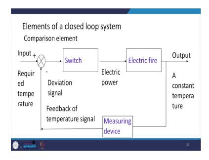
Now, if we talk about the closed loop one; then what we do here is that, form an electric fire or the output, we take that output through a measuring device and feedback this temperature signal to the comparison element, where the input that is what require temperature we want that is and the feedback is compared and a deviation signal is found and that deviation signal is given to the switch and again that switch supplies power to the electric fire.
