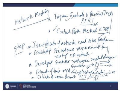
So, there are various techniques which are used in network modelling. The two are of the great importance and which are extensively used. One is called Program Evaluation and Review Technique. In short, it is termed as PERT.
