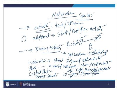
So, for developing any network we use symbols. Symbols are basically in form of the arrow which is showing the activities or which is say, required to be done for completion of the project or you can say many activities will be required to complete the project so these will be shown by the arrow. Then there is a node or event. An activity will always have a kind of nodes at the beginning and at the end.
