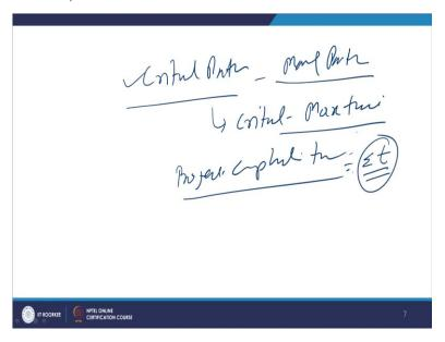
Then the critical path. A network may have many paths. In a network there can be many paths but the path which takes the maximum time to complete is termed as Critical Path. I will give the example. Critical Path, one which takes the maximum time for completion of the activities falling on the critical path.
