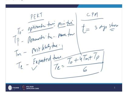
Say, in case of the PERT approach, the time is expressed in different way than in case of the CPM approach. So, in case of the CPM with the great clarity, that the expected time, the time particular activity will take is known with the greater clarity. So, we will write clearly like it will take 3 days or 3 hours.
