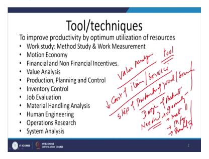
Then we have the value analysis. This is the kind of a tool or technique which is available in the industrial engineering with the goal of reducing the cost of the item being produced or the cost of the service or the cost at which service is being provided. In this approach, each step of production, of goods and service, not just production, but the design of the product is challenged to see if it is a really needed or not.
