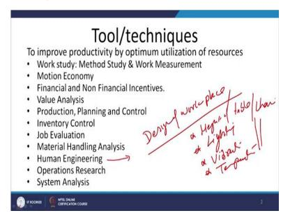
Another aspect that we look into the human engineering is the design of workplace like what should be the height of the table? What table, what should the height of the chair, how the, what kind of the lighting should be provided during the work as per the kind of the size of the equipment to be handled.
