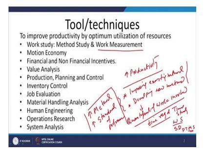
Starting with the work study, what we have work case study is a tool available in industrial engineering which helps in basically increasing the productivity. And for increasing the productivity it uses the two approaches; one is called method study, which helps in improving the existing method of doing the job or developing the new method. Idea behind this is that all the non-productive elements are eliminated and the job is done in most efficient manner in the minimum possible time.
