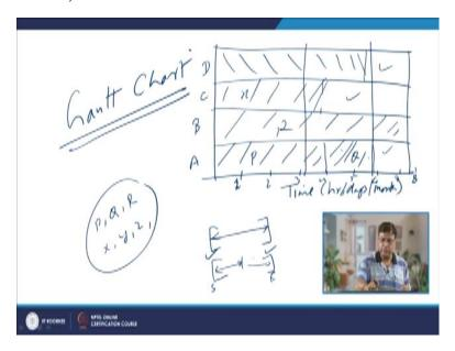
So, we will be starting with the Gantt chart. So here, Gantt chart is basically a simple chart only where we basically indicate, in y axis we indicate the time, this time can be in hours, can be in days, can be in months. And then in y axis we can mention the jobs. So, here 1, 2, 3, 4, 5, 6, 7 like this, we can mention like 1, 2, 3, 4, 5, 6, 7, 8 and then in y axis we can have number of subjects, which may be in form of the operations to be performed or the worker who will be doing the job.
