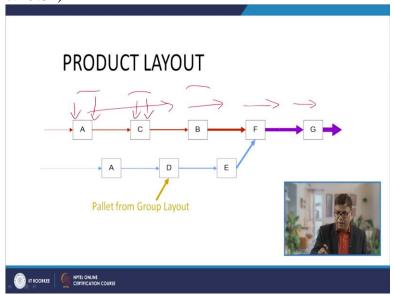
Let us see, the little bit details of, in the typical product layout what we have? Like say, the equipments are arranged in the sequence of the operations to be done. And the, these are designed in such a way, the activities to each station is assigned in such a way that they take almost equal time to complete, so that the wastage of the time at each station is minimized. And there is no backtracking and streamline movement.
