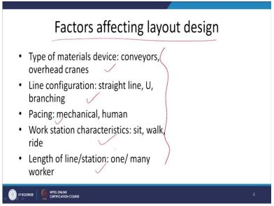
About this I have already talked like, how can we understand the different kind of the product layout designs, depending upon the kind of the facilities which are being used to move the material as per kind of the material handling device, kind of the configuration of the line which exists, the way by which the material is moved, the station characteristics and the kind of the length of the line, or the station where we are deploying either one or the number of persons.
