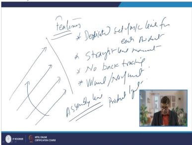
So, as far as the features of the product layout are there which will be affecting the design, like dedicated set of the machines, which means dedicated line for each product. Then there is the straight line movement, straight line movement, always movement, straight line movement so there is a clarity in the direction in which, regarding the direction in which the movement of the material during the processing will be taking place.
