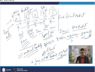
So, the typical arrangement which is used here is like there is a set of the facilities. Like say there is station A, Station B, station C, Station D, Station E. So here what do, basically the raw material is fed in. And after getting processed through the different stations; at the end we get the final product.
