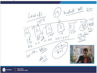
So here, if we see the line efficiency is the another thing, line efficiency. Say, in a line there are 5 stations, A, B, C, D and E. And for a given production rate, let us say cycle time is 2 minute, and what we see that the job at station A is completed in 1.8 minute, job B, at station B job is completed in 2 minutes, at C it is completed in 1.4 minutes, at D it is completed in 1.9 minutes, and at E say it is completed in 1.5 minutes.
