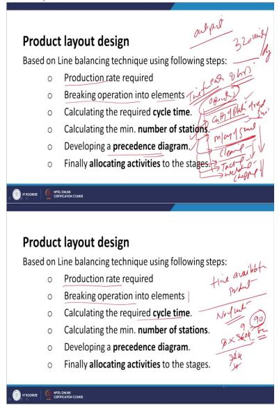
What we have to consider here, for designing the product layout, the basic method in designing the product layout is the balancing of the line. Which means the different stations are designed in such way, that all will be having the almost equal time required to complete the job at each station, so that the wastage of the time at each station is avoided or minimized.
