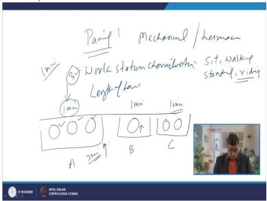
So, then we have the how the material is moved. So, how the pacing is done or the material is moved, so it can be mechanical or through the human effort. Then the work station characteristics. Like the worker will be sitting while work is being done, or worker will be walking during the operations, or he will be standing during the operations, or he will be riding on the belt during the, belt or the material handling device during the work.
