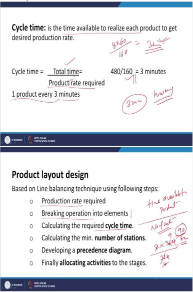
So here, if we see just for clarity. Cycle time is the time available to realize the each product to get the desired production rate. So, the total time available and the kind of the production rate which is required, the production rate which is required. So here in this case, say the total time available in 8 hours, 60 minutes and if the desired production rate is 60, so the 3 minutes becomes the cycle time. We cannot allow the time to complete the job at each station more than 3 minutes.
