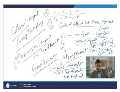
So, considering this cellular layout, this is also called the group technology layout. In this case, as name appears, the cellular layout basically we create the cells of different sets of machines equipment and facilities. So, cell one will be of one type, cell two will be of the second type, like this and each cell is made independently to perform certain types of jobs.
