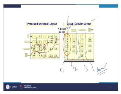
Now, here we see, if we take the example of the manufacturing of the components like a ring, the shaft with the whole or the shaft having steps or this rectangular component with the whole. So, the kind of if the, if these four components are manufactured using the facilities having the arranged according to the process layout.
