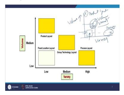
So where, so how to choose the suitable type of the layout as I have said, when extremely high variety, so there are two factors like we can have like if the variety in X axis and the number of units or volume to produce in Y axis, then for extremely high variety and very low volumes like in batch production, we try to have the process layout.
