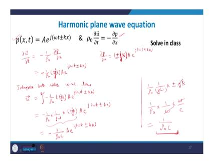
So, p function is known to us and this is the equation through which we will get the function for the velocity. So, let us say del u by del t is equal to minus 1 by rho naught del p by del x. And del p by del x is what? Del p by del x is going to be; if we differentiate this you will get plus minus k times of A e to the power j omega t plus minus k x
