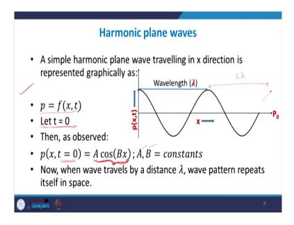
So, here we use this assumption. So, a simple harmonic plane wave; that is traveling in the x direction that is the equation we want to get. Now, we know that this wave will be a function of both space and time. So, it will be p x comma t. So, let us see here. So, this p is a function of both space and time. So, let us first freeze the time and see how does it vary over space.
