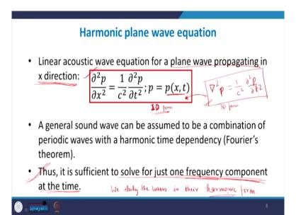
So, let us derive the equation for a harmonic plane wave. So, here we will derive the equation for a harmonic plane wave. So, we have already seen the equation that is nabla square p is equal to 1 by c square times of del square p by del t square. This was a general equation for sound wave propagation in fluids. And now, here let us say the plane wave is propagating along the positive x direction and the direction in which the plane wave propagates.
