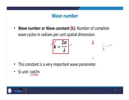
So, wave number or simply the wave constant is represented by the symbol k and mathematically it is 2 pi by lambda and it is defined as the number of complete wave cycles in radiance per unit special dimension. Which means that; if you take 1 meter. So, within a 1 meter of space how many 2 pi revolutions that particular wave is making. So, this is given by 2 pi by lambda. So, again the S I unit of this is radians per meter.
