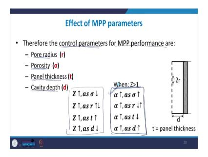
So, now we already have this the control parameters that we have found for MPP are pore radius, porosity, panel thickness and the cavity depth. So, it depends on all these 4 properties. So, the Z depends on these properties and we found this is the kind of relationship and because we are taking this particular case because for most of the cases 99 percent of the cases MPP will have an impedance more than that of air.
