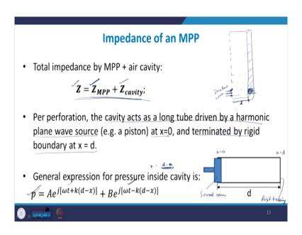
So, if you begin first, then this is the this is giving us the acoustic impedance of this micro perforated panel, but the micro perforated panel also has a cavity behind it. So, that together the impedance of the material will then be the impedance or due to the micro perforated panel plus the impedance due to this cavity. So, this will be the total acoustic impedance. So, what
