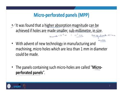
So, to begin I will like to say what is a micro perforated panel. So, it is same as in the case of a perforated panel absorber, but the limitation in perforated panel absorber was that the absorption magnitude. So, both for Helmholtz resonator and perforated panel absorber because they both are based on the same principles of Helmholtz resonance.
