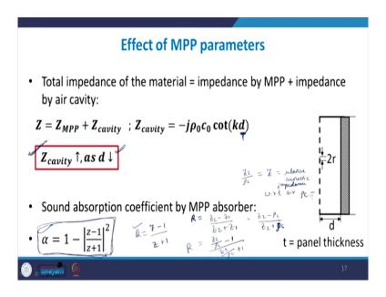
So, the first control parameter. So, control parameters are those parameters in the design of an MPP that will change its acoustic impedance. So, the first parameter that affects the acoustic impedance of this particular material is going to be the cavity depth because Z of cavity depends upon the cavity depth. So, depth of cavity so obviously, the Z will be dependent on the target frequency; but other than that, what are the design parameters on which it depends?
