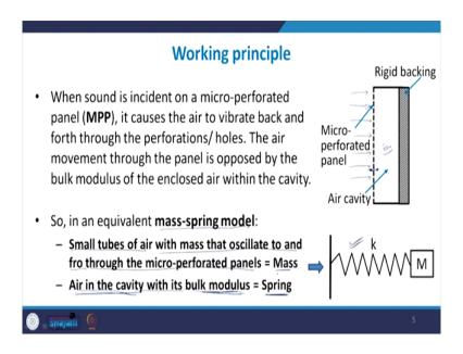
So, this is again a special spring type of air spring oscillator just and it works like Helmholtz resonator. So, as I have explained. So, I would not go to the detail of the working principle here because it is the same as the perforated panel absorbers. So, effectively what happens is that when the sound energy, it is incident on these panel, then it and then this panel itself will have its own resonance.
