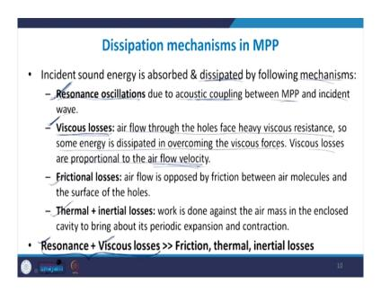
So, the various mechanisms operative here for dissipating the sound energy are first of all it is the sound energy is lost at the resonance because the acoustic coupling takes place between the MPP and the incident wave and then, the energy is now being used to do work in driving the; driving the MPP at resonance or driving the air molecules or oscillating them at resonance.
