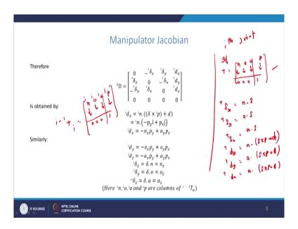
Now, if you recall the formula; D superfix T is given by this expression ah; del z t and del y t etcetera; where in the place of T we are putting i because it is corresponding to the ith joint. The differential changes corresponding to the ith joint is given by this one; so we are indicating this superfix i at every place.
