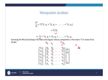
So, now we recall the other formula d T by d small t is also same as T into D superfix T ah; where the D superfix T are the differential changes with respect to the current frame. So, the differential changes with respect to that current frame is given by the differential changes with respect to the first frame; that is D 1 T and the differential changes with respect to the second frame D 2 T etcetera; where the general D i T is given by this particular formula here.
