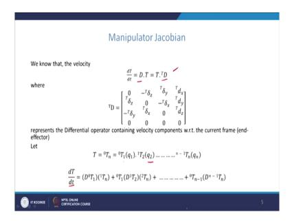
So, now we have already seen this particular formula; that is the velocity of the frame T is given by D into T; where D is the differential changes or the velocity of the frame with respect to the base frame D; base frame the 0th frame.
