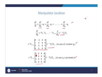
So, we will write it in the following way; del T by del q 1 into d q 1 by d t plus del T by del q 2 into d q by d t etcetera is the standard formula of the total derivative using the partial derivatives.
