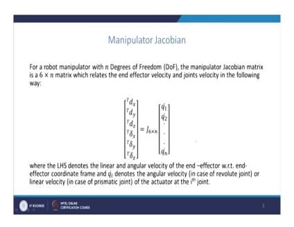
It is a relation which relates the d x T, d y T etcetera and del x T, del y T, del z T; these are the differential changes; the linear changes, the first three one along the x y z direction of the current frame that is the end effector frame and del x, del y, del z superfix T; they are the differential rotations about the x y z axis of the end effector frame; so that is the left side.
