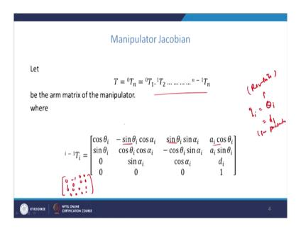
So, the end effector 0 T n is given by the product of 0 T 1, 1 T 2 etcetera as we have seen the previous slide. The ith frame with respect to i minus 1th frame is given by this expression.
