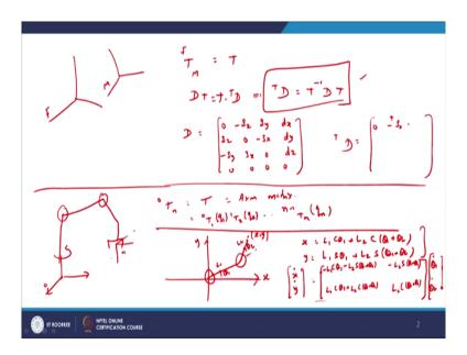
So, we have seen the following that if you have two frames a fixed frame and a moving frame and if the relation between F and M; that is M with respect to F is denoted by the homogeneous transformation T.
