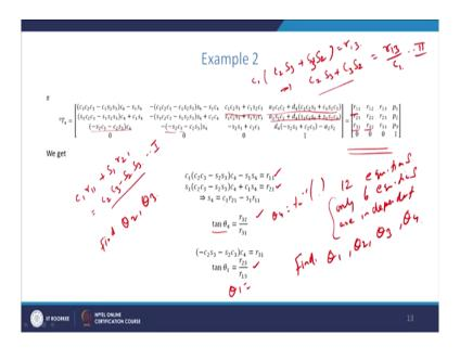
Now, if we are given a specific 4 by 4 matrix representing the end effector position like this n o a p matrix. Then we can directly equate each terms here, we can easily see that even though there are 12 such equations. There are 12 expressions here and in the right hand side corresponding 12 numbers are there. So, if we equate there are 12 such equations, 12 equations are there.
