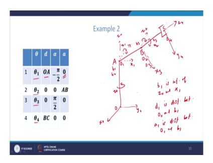
So, in the first example we will see a 3 degree of freedom manipulator and then in the second example we will see a 4 degree of freedom robot manipulator for which we will construct the kinematics equation and then the inverse kinematic solutions.
