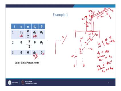
So, for this first example; we see the following robot manipulator. So, we consider a platform in which the axis of rotation is the vertical direction; we call it as the z 0 direction. So, the entire platform rotates in the horizontal plane with the vertical line as the axis of rotation. Then the robot manipulator is placed here. The stem of the robot manipulator is placed here for which there is a joint which rotates with the axis of rotation perpendicular to the plane of the paper.
