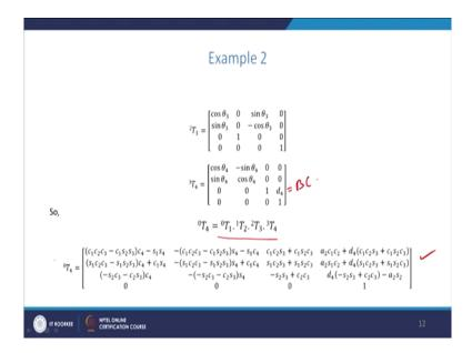
Now, substituting all this values in the product we finally, obtain the direct kinematic problem the equation 0 T 4 is the end effector position with respect to the base of the manipulator.
