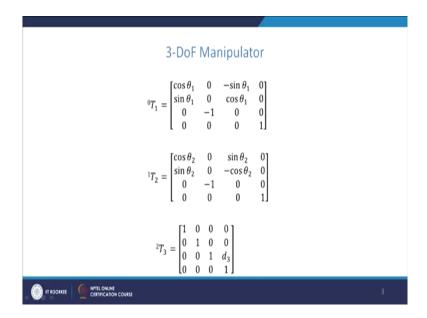
0 T 1 is given by this expression and 1 T 2; for 1 T 2 we should substitute the values of the parameters theta 2 and alpha is pi by 2. If you substitute we get the second 1 T 2 matrix and 2 T 3 is given by the third one. If we substitute d 3 is the distance o b. So, that expression is given by and theta is the angle 0 in this case. If you substitute here, we get the identity matrix for the first 3 by 3 matrix and 0 0 d 3. So, these three matrix give the joint coordinate systems.
