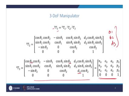
Now, if you multiply all these three we get the 0 T 3 homogeneous transformation, which gives the end effector coordinate frame with respect to the base coordinate frame 0. So, the product finally will give 0 T 3 is given by the expression given here in terms of theta 1, theta 2 and d 3. These are the three variables: theta 1 theta 2 and d 3 variables are there.
