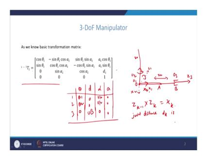
So, as a first example we see a 3 link manipulator in the; as shown in the following picture. So, the manipulator is having the axis of rotation is the vertical axis and one horizontal axis which is perpendicular to the plane of the paper. So, we call this as the Z 0 axis and the perpendicular to that as the Z 1 axis. So, these are the two degrees of freedom situated at the single joint, we call it as O. Then the robot manipulator if it is in this form let us assume that.
