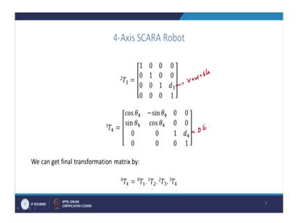
And d 3; d 3 is a variable, because the third joint is a prismatic joint it is varying from the value. That is the lowest value is 0 and the highest value is the length of that particular link. The maximum length of the link can be the highest value for that variable So, now d 4 is the final this thing this is DE, up to the end effector to the previous link. So, these values can be substituted and by multiplying the four matrix: 0 T 1 1 T 2 2 T 3 and 3 T 4 we get the end effector position.
