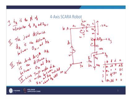
So, here we consider a 4-Axis SCARA Robot manipulator. So, the manipulator which we will consider is the following. We consider the this is revolving about the axis, z axis z 0 axis is a vertical line and so this joint is a fixed one, there is no movement at this joint. We call the base as o and this joint as A where there is no movement it is 90 degree l shaped position.
