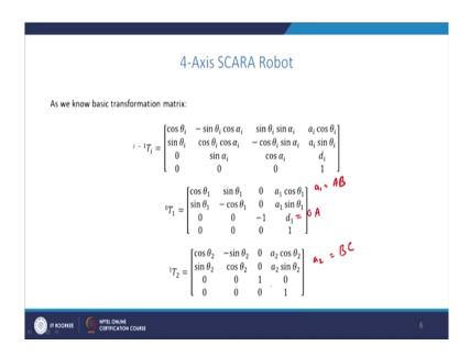
So, what we observe is 0 T 1 when we substitute theta 1, for d 1 we substitute o A that length. This is actually, so first joint this o A. So, the first joint distance d 1 is o A. So, we substitute in the place of d 1 this one. And a 1, in the place of a 1 we substitute the distance AB; whatever is the length AB. Similarly for A 2 we substitute the length BC depending on the size of the robot manipulator.
