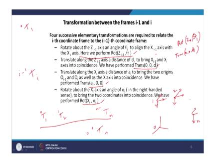
So, if we have the base coordinate frame like this and another coordinate frame to be like this and the third joint has a coordinate frame this way and the end effector coordinate frame is this way. So, we can have the 0 th frame and then first frame second frame etcetera the nth frame we want to find the relation between the first frame with respect to the 0 th frame and
