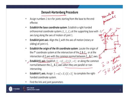
So, first let us see what is the D H procedure; Denavit Hartenberg procedure. So, first we have to assign the numbers for the joints. So, we can call this as the first joint is the base that is 1 then 2, 3, 4; the end effector is 5; in this particular picture we say there are 5 joints. Now
