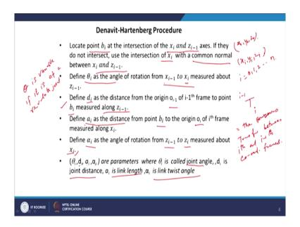
So, using this coordinate systems, next we can find the relation between the i th coordinate system and the i minus 1 th coordinate system so, we want to see. So, now we give the coordinate system as x 0 y 0 z 0 is the base coordinate system; x i, y i, z i is the i th coordinate system. i is equal to we can have 0, 1, 2, 3 up to n; n'th coordinate system is the end effector coordinate system. So, by D H procedure, we have already fixed this coordinate system.
