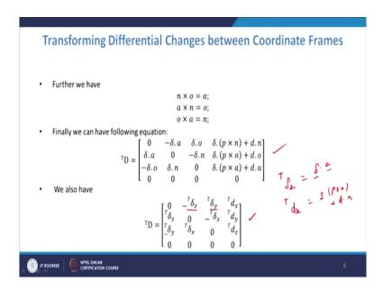
So, what we ultimately obtain is the d super fix T is given by this matrix 0 minus del dot a del dot o del dot p cross n plus d dot n etcetera. So, it is a very straight forward simple formula, which is relating d super fix T and the D matrix.
