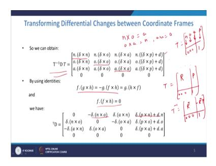
Now, we have to multiply in the left side T inverse. So, T inverse D T can be obtained like this, it is because the T inverse if T is given by the rotation matrix the 3 and then P vector 0 0 0 1, where R contains the first row is first column is n o a and then this is p as shown earlier. So, the T inverse, if you recall it is nothing, but R transpose the 3 by 3 matrix and minus R transpose into p vector then 0 0 0 1.
