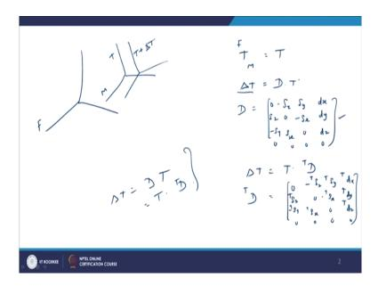
So, to recall that one, if you consider a fixed coordinate frame F and another coordinate frame M, then if you write the frame M with respect to frame F, that is F T M as the homogenous transformation T. The positional orientation of M frame with respect to F frame is given by the 4 by 4 homogeneous transformation matrix T. And then and if we give a small translation and rotation with respect to the fixed frame, then the new position of T will become T plus del T.
