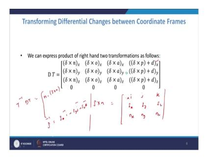
So, that is the first element of this product. And that can be easily seen to be the ex component of the del cross n, this del cross n, it is given by del x i j k, del x, del y, del z n x, n y, n z. So, this determinant if you calculate the ith component is del y n z minus n y del z. So, that is what we have seen here this one. So, this is the first component del cross n x.
