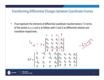
So, we denote this F T M the M frame with respect to F frame by the 4 by 4 matrix like this, where the first column represent the n vector o a p the some standard notation for the 3 4 columns of the homogeneous transformation.
