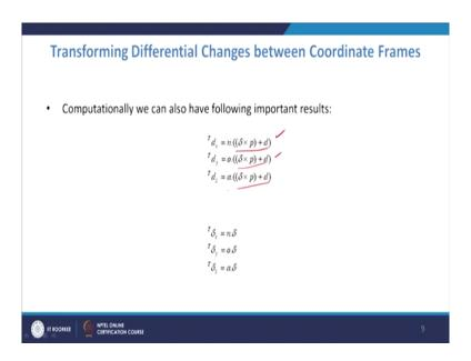
And then we can take this n as a common factor, we can get the res the result like this. Del cross p plus d is a vector which we can calculate and then if you take with the dot product with n that is the linear velocity, along the x direction dot product with o will give the linear velocity along the y direction of the current frame etcetera.
