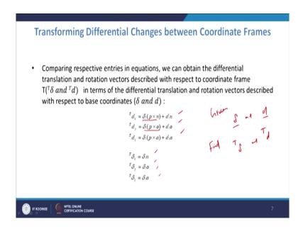
This gives the formula that the these are the linear velocities and then these are the angular velocity. So, what is important in this formula is if we know del and d. If it is given; that means, the translational velocity and rotational velocity with respect to the fixed frame, if it is given, then we can find the translational velocity and rotational velocity with respect to the current frame.
