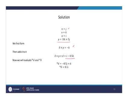
So, that is calculated by this as formula as given here. So, here n matrix is the first column; first column is 010. So, it is j and the o second column is k vector and the third column is i vector and fourth origin is shifted to 10 i plus 5 j position. So, and the del cross p is calculated where del is given by this one, this in vector and d is given by this. So, del cross p can be calculated, del cross p plus d is finally, this one this transformation.
