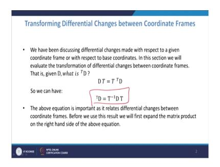
So, here D into T is same as T into D super fix T as seen in the earlier slide. So, D super fix T is given by this formula that T inverse D T. So, if you are able to evaluate this expression in the right hand side expression we get the relation between D and D T. And then we can make use of the many certain problems.
