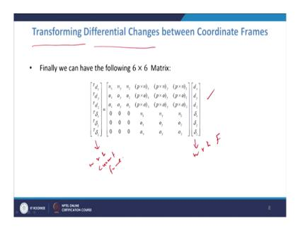
So, now if we summarize this in a matrix form we get here d x, d y, d z r this is with respect to the fixed frame and we can find it with respect to the current frame. So, this formula is a useful one to which is relating. So, it is the transforming the differential changes between coordinate frames F frame and M frame, we are transforming it and this formula is useful in that context.
