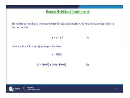
Assuming that our model of friction is a function of joint positions and velocity, we add that term which is the  $F(\theta, \dot{\theta})$  two equation 1 so, that the model we obtain is will be
