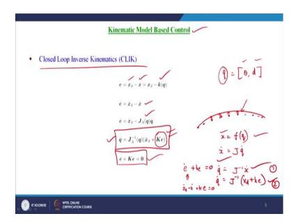
Now, coming to the control based on the model of the manipulator, thus model based control first we discuss about kinematic model based control. It is nothing, but closed loop inverse kinematic scheme. Because we ensure that the error goes to 0 as the time tends to infinity by a first order dynamic equation.
