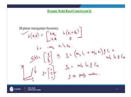
So, the  $M(\theta)$  part that the inertia matrix part is over, now coming to the matrix  $v(\theta, \dot{\theta})$  which is nothing, but the matrix which involves the Coriolis and centrifugal efforts which is given by
