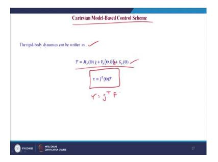
Then we come to Cartesian model based control scheme. So, far we have seen joint space model based control scheme and this is what Cartesian model based control scheme. So, the rigid body dynamics can be written as
