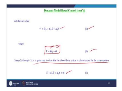
With the servo law, we have the servo law considered so, that the feedback from both velocity of the joint trajectory also the position of the joint trajectory error is considered in the servo law. So, that  $\tau'$  is servo law given by
