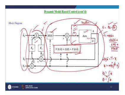
Now, coming to the block diagram, explaining or schematically representing the dynamic model based control scheme is shown here, where we give the joint trajectories as the input
