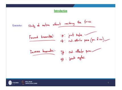
Now, coming to the introduction, first we talk about kinematics what is kinematics? Kinematics is the study of motion without considering the forces associated with. Kinematics can be classified the robot kinematics can be classified into forward kinematics, which is the input is joint angles whereas, the output is end effector pose which is nothing, but position and orientation. Whereas, inverse kinematics that is nothing, but the input is end effector pose and the output is joint angle.
