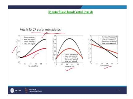
And we have simulated this for a two link revolute planar manipulator with this model based control scheme, for the given decide joint trajectories of the two joints. So, we have from the controller, we have obtained that the joint trajectories decide joint trajectories have been exactly matched by the control scheme involving the dynamic model.
