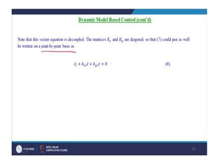
Note this the matrices  $K_v$  and  $K_p$  are diagonal. So, for a joint by joint basis for the joint i that aerodynamic equation can be written as
