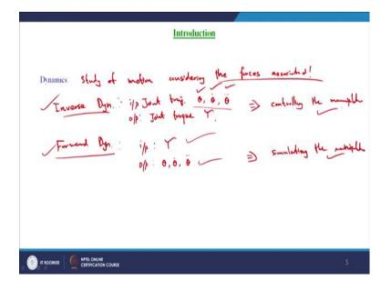
Now, coming to the dynamics portion what is dynamics? Dynamics is the study of motion considering the forces associated with that motion. Dynamics can be further classified into inverse dynamics and forward dynamics. What is inverse dynamics? Inverse dynamics the input is joint trajectories in terms of  $\theta$ ,  $\dot{\theta}$ , and  $\ddot{\theta}$  position, velocity and acceleration of the joint angles and the output is this is the input is joint trajectory, the output is joint torque.
