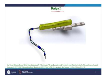
The design 2 states that it has four degrees of freedom; the first degrees of freedom is the translation motion which is done by this rack and pinion system and then it has revolute joints which are realizable by the SMA wire actuators attached to the lateral side of the needling system. So, this is the cad model which shows the design 2 which we have developed in our lab and this is the reference of this work is given in this citation.
