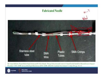
Now, this is the fabricated needle which we have developed. So, as to have a smart actuation, so that the target is reached with the contour shape over the needling shape of the path.
