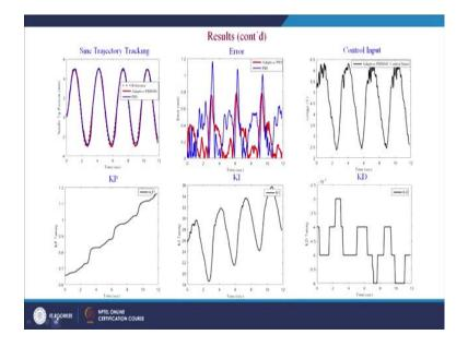
So, we have given the sinusoidal trajectory. So, that the needle can take the continuous trajectory as shown here and the error for that is given in this figure 2, where the control input is shown in figure 3. And corresponding  $K_p$  tuning value  $K_p$ ,  $K_i$  tuned value and  $K_d$  are shown in this figures which are varying between 0.6 to 1.24  $K_p$  and 8 into 36 for  $K_i$  and it is varying in the range of 10 power minus 3 for  $K_d$ .
