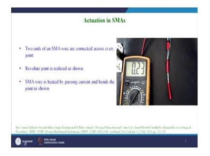
How the actuation is done for the needling system through the SMA wire is shown here. As you can see that by passing current through this lateral side SMA actuators we can have this bending degrees of freedom which is what is shown here is the revolute joint is realized by passing current through the lateral side SMA actuators.
