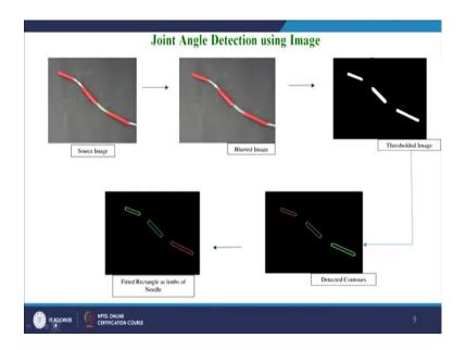
Precisely this is what happening; first the source image which is the RGB then we blurred it then we get the threshold image, which is basically a binary image then we detected the contours which is not exactly rectangular in shape. So, we made it rectangle by fixing a rectangular shape on the contours successive contours, then we got the joint angles between the successive. So, this way we can find the joint angles this is  $\theta_2$ , this is  $\theta_3$ , this is  $\theta_4$ .
