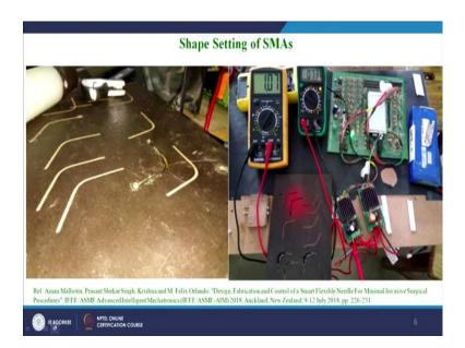
Now, coming to the shape setting of the SMA actuator wires. We have chosen the nitinol wire actuators, so that it gives more pulling power compared to the other forms of SMA
