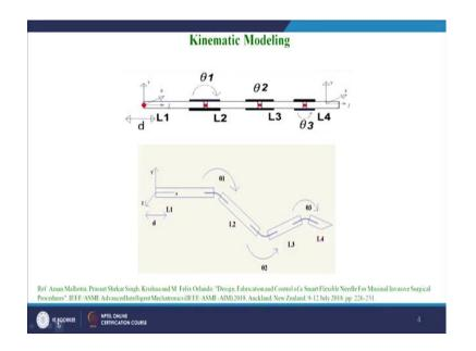
Now, coming to the kinematic modeling of the design 2 smart needle, it has four degrees of freedom. First being the translational degrees prismatic joint based. So, that the whole needle is pushed forward or pulled backward and the second degrees of freedom is a revolute joint which has 2 SMA wires attached on the lateral surface.
