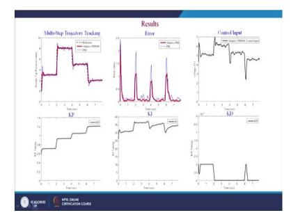
Now, coming to the results associated with this work we have performed the analysis through multi step trajectory tracking. First we have given the multi step trajectory, we have first given started with 4, 3 millimeter, then we started with 8 millimeter, then we have given another random step then again a random step.
