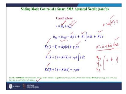
So, the sliding mode controller is having the two parts; first part the second part. Where the first part is the discontinuous part which is given by  $ksat(\sigma)$ , where  $\sigma$  is the sliding surface which is given by  $\sigma = \ddot{e} + k_1 \dot{e} + k_0 e$ . So, this is the sliding surface which we have considered in our study and how and why this has been taken has been given in this reference clearly.
