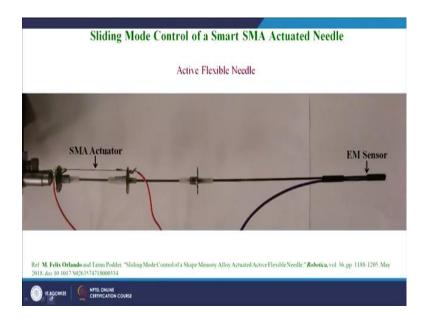
So, now coming to the robust control of a smart SMA actuated needle. So, this one we have done in order to see that the disturbance given to it can be overcome or not. Because of once the needle is inserted into the real tissue there could be lot of disturbances coming to the needle and how the needle is going to face that and overcome those disturbances.
