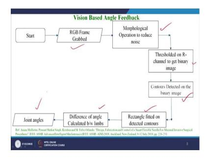
Now, coming to the vision based angular feedback. So, we have seen the bending of it and we want to grab that actual angle of the bending of the needling system by a vision camera system a vision system; which is here stereo camera system to get the bending angle of the robotic smart needle.
