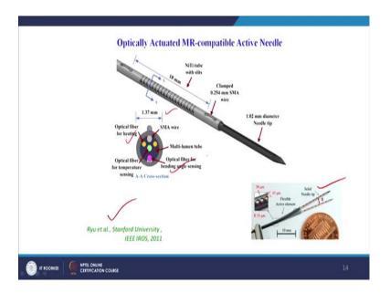
And the other needle design is proposed by Ryu et al from Stanford University. So, he has proposed the system which he is shown here which is of precisely good size here which is a smaller size. So, it has been used for it will be used definitely for the surgical purpose for conventional cancerous percutaneous interventions. It can be used for the clinical procedures and this outer dia of the needle is such that it is 1.37 millimeter dia.
