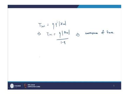
Thus we have proved that both convergence of distance as well as convergence of time for the state variable trajectory in this higher order sliding mode which proves finite time convergence.
