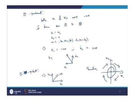
Next, we go to the III quadrant; what we have is both  $x_1$  and  $x_2$  are negative. So, from equations 1 to 3 which is  $\dot{x}_1 = x_2$  and  $\dot{x}_2 = u$  and u equal to
