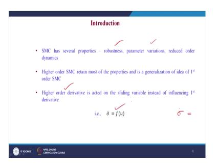
Coming to the introduction; sliding mode control has several properties, finite time convergence, robustness, parameter variations, reduced order dynamics. The higher order sliding mode control retain most of these properties and is a generalization of the first order sliding mode control. Here in this higher order sliding mode control, higher order derivative is acted on the sliding variable  $\sigma$  instead of influencing first order dynamics.
