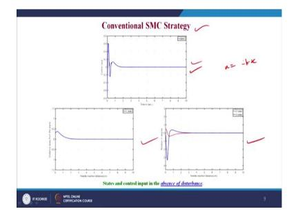
So, here we see the conventional sliding more strategy without the presence of disturbance. So, this can be the same system performance the evolution of the states and the control input without a chattering can be observed by a simple state feedback controller u = -kx can also be used to observe this because there is no distance disturbance in this control problem.
