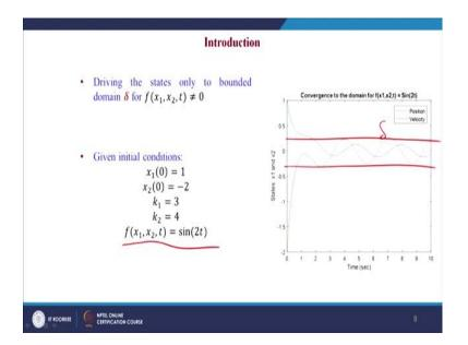
And, what happens when the disturbance is given that is  $f(x_1, x_2, t) = \sin(2t)$ . When this disturbance is given that straight feedback controller will make the system states common state or stay in this domain, which is this domain is delta which is a function of  $k_1, k_2$  and the bound value L. It is not getting converged whereas; it is going to this domain and stays there by this control law.
