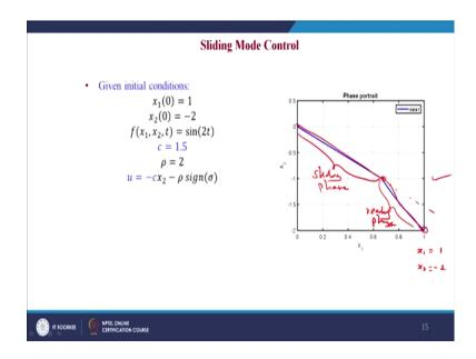
Next we are seeing that convergence of the state variables from the initial case  $x_1(0) = 1$  and  $x_2(0) = -2$ , we have from started from this trajectory that is the reaching trajectory after reaching it goes to the sliding surface, that is here this phase is called reaching phase of the system states. And, this phase is called sliding phase of the system states.
