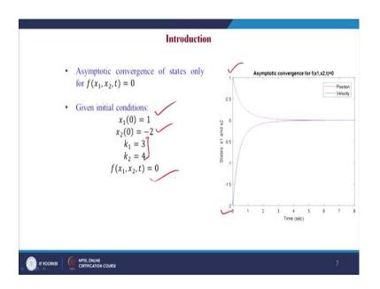
Consider the example which is the single dimensional motion of the mass with states position and velocity with the given initial conditions,  $x_1(0) = 1$ ,  $x_2(0) = -2$  with the controller gains  $k_1 = 3$ ,  $k_2 = 4$  respectively. And, with the disturbance being 0 it will converge the system to stability to equilibrium point at time tends to infinite, that is the asymptotic convergence for the system is obtained for the disturbance being 0 by this state feedback controller.
