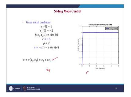
Next what happens to the state to the variable that is a sliding variable? How it is converging in the time domain? We are seeing in finite time convergence, as you can see that it is getting converged in the finite time to 0. The sliding variable sigma is converged to the equilibrium point 0 at the finite time  $t_f$  which is much close to 0.25 seconds as can be seen here in this figure.
