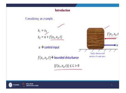
Considering an example of single dimensional motion of a unit mass as shown in the figure here, which is pulled by the control input force and which is resisted by the disturbance force which is given by the term  $f(x_1, x_2, t)$ . Where the disturbance is a bounded disturbance and this disturbance has is including the viscous friction force as well as the unknown rigid forces associated with this mass and the system states are  $x_1$  and  $x_2$ .
