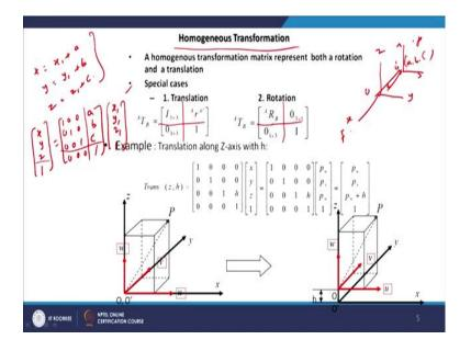
So, now we consider the homogeneous transformation. So, so far it was considered only about the rotation, rotation about x y z axis or rotation about any general axis, but if the coordinate frame is translated that is a fixed frame F is given and if the origin is shifted to some other position without disturbing the directions of the three axis x y z axis are kept parallel all the time and only origin is shifted to a different position in that case the motion is called a translation.
