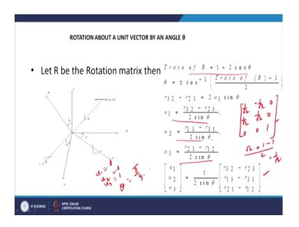
So, now we will see this structure is useful in identifying the amount of rotation and about which axis a rotation is performed. So, for example, a arbitrary rotation matrix is given. So, earlier we have seen that a rotation matrix is a orthogonal matrix in addition to that it should form a right handed system. So, if you give a rotation matrix, then how to identify the axis of rotation as well as the amount of rotation. So, for that it will be very useful.
