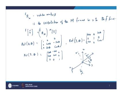
So, in the last lecture the notation  $FR_M$  was introduced which represent a rotation matrix; it represent a rotation matrix and it gives orientation of the M frame with respect to the F frame. So, it gives the relation between a coordinate the coordinate of a point r and the coordinate of the same point with respect to M how they are related. So, this  $FR_M$  represent the matrix relating the M frame with respect to F frame.
