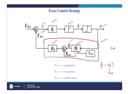
So, the block diagram associated with the proposed control strategy of the force is given by, given the desired force may be a scalar or a desired trajectory it works for both. So, we considered first with the scalar that is a set point, then we can also implement a desired trajectory. So, given the desired force it is multiplied with the gain matrix, so that Jacobian transpose comes into picture.
