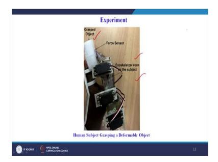
Schematic shows that experimental model or experimental exoskeleton own on the human subject grasping a deformable object. Where the force sensor is attached to the surface lateral surface of the body of interest to be grabbed and the exoskeleton master may the slave human subject finger in order to grab the object with the desired force of interest.
