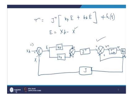
So, when we have the impedance control implemented on the manipulator, the control law will take the form  $\tau = J^T [k_p E + k_d \dot{E}] + G(q)$ . Where the error E is given by
