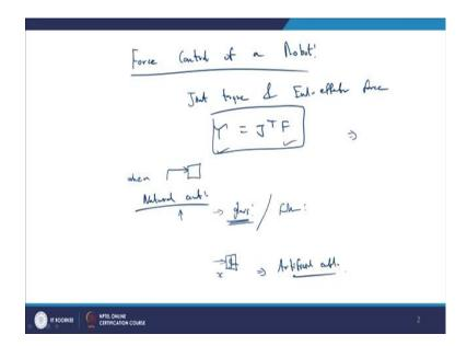
Coming to the introduction. So, force control; so force control of a robotic system. So, before that we should know how the joint torque and the end effectors force. Force are related that is by the static relationship  $\tau = J^T F$  we can have this relationship between the joint torque and the end effector force through the Jacobian transpose relationship.
