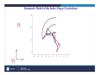
The kinematic modeling is observed in such a way that we have simulated. So, that the serial attachment by the former kinematic equation is providing the moment in such a way that this type of simulative trajectory can be possible. As you can see that the magenta line shows the trajectory of the end effector and the red line shows the trajectory of the middle phalanx 4 bar and also the second red line shows the territory of the proximal fellings of the index finger part of the exoskeleton.
