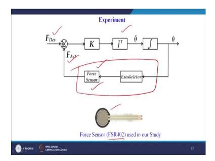
So, we have performed the experiment by having the desired force given, with the actual force obtained through these sensor feedbacks. Where the sensor is a force sensor which is basically FSR 402, sensor which is giving the force value based on the resistance value change this is the force sensor which is attached to the body surface.
