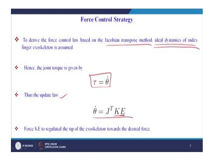
Now, coming to the force control strategy associated or proposed in this study is that transpose of the Jacobian method is utilized. So, that the ideal dynamics of the index finger exoskeleton is assumed. Hence the joint torque by the ideal dynamics is given by tau equal to theta dot, with the update law being  $\tau = \dot{\theta} = J^T KE$ . Thus the force which is given by the product of K with the error is used as a regulating force for the tip towards the desired force.
