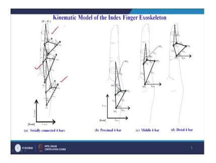
The kinematic model of the index finger exoskeleton shown here with the perspective that 3 robotic 4 bar mechanisms are serially connected. First one for the proximal phalanx, the second one 4 bar for the middle phalanx and the third 4 bar for the distal phalanx connected serially. So, that they form the index finger exoskeleton for the moment of the index finger.
