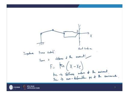
So, now let us consider a manipulator, where the tool is in contact with the environment which is basically the hot surface X direction, point P is the point of contact and thus the manipulator with its end effector having the tool. So now, when we see through the impedance force control, we observe that there is stiffness of the environment. Through this control what we observe is we have the stiffness of the environment which is used to control the tip on the surface through the force control.
