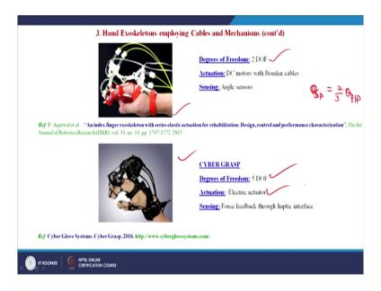
In continuation with the exoskeleton see employing cables and mechanisms. This is the exoskeleton proposed to by Agarwal et al and it has been published in the I J or journal in the year 2015 and this is the exoskeleton which has 2 degrees of freedom this is here shown only for the index finger. It has 2 degrees of freedom one for the flexion extension of the MCP joint and the other degrees of freedom other motor is for the collective or the coupled motion of the PIP and the DIP joint.
