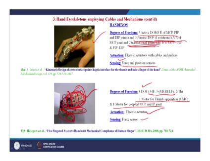
Then we have the hand exos proposed by the author I could not remember. So, this author has proposed this hand exos exoskeleton which has degrees of freedom 3 that is active 3 degrees of freedom that is for flexion extension of the MCP joint P I P joint and the DIP joint and 3 passive degrees of freedom. That is, 1 rotational degrees of freedom that is passive 1 rotational and 2 translational rotational translational degrees of freedom.
