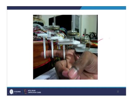
So, with that notion; we have developed the 4 bar based exoskeleton which will be discussed in the next lecture. Here it shows the index finger exoskeleton which is having the 4 bar mechanisms connected serially from the base till the distal part of the index finger and the conclusions coming to the conclusions finally with this lecture.
