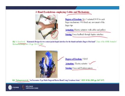
Now, coming to the third and the final classification of exoskeletons implying both the cables as well as the mechanisms; first is the model proposed to by Frisoli et al in the year 2007. So, here you can see that the degrees of freedom for this exoskeleton proposed is 6 degrees of freedom to track any movement of the fingertips, 3 for the index finger and 3 motors for the thumb.
