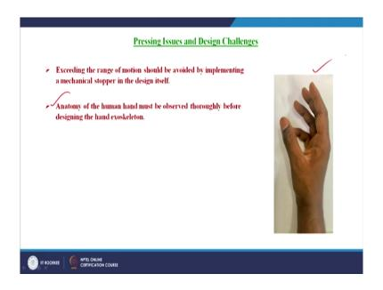
And another thing is; the range of motion must not be extended and it must be avoided by a mechanical stop by a simple mechanical stopper in the design itself. Then finally, the very important thing is; the anatomy of the human hand must be observed thoroughly before designing the hand exoskeleton. As you can see that the hand exoskeleton the hand the human hand forgot. First, we considered the hand in such a way that coming to the anatomy of the
