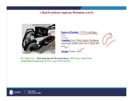
Now, coming to the fifth type that is the latest model which has been developed is the one which is the hand exoskeleton which has 3 degrees of freedom for each finger using only mechanism. They have used a mechanism with your series elastic actuator such that both
