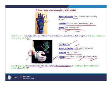
Then in continuation to the hand exoskeletons employing cables; we have the another exoskeleton which is recently developed in 2017 by Popov et al which is a portable exoskeleton in order to perform activities of daily living such as grasping and object manipulation. So, it has a degrees of freedom it is basically a glove type and it is basically has 4 degrees of freedom excluding the little finger here.
