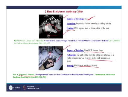
Now, coming to the second category of hand exoskeletons that is first done by Di Cicco et al and this is the one has been developed in the Carnegie Mellon University. And, this exoskeleton is a one which is actuated by pneumatic pistons via a cabling system and it has 2
