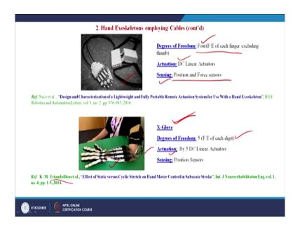
In continuation to the hand exoskeletons employing cables; we have the one which is proposed by Nyez et al. And, this is the exoskeleton which has a degrees of freedom 4 that is accept the thumb actuating the four other fingers index finger middle finger ring finger and the pinky for natural flexion extension of each finger. And, the actuation is done by linear actuators D C linear actuators.
