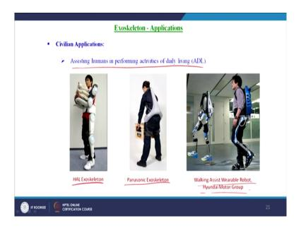
Finally, the civilian applications there are these exoskeletons are developed in order to assist humans in performing activities of daily living like lifting, walking and performing personal tasks such as writing and opening the knobs etcetera.
