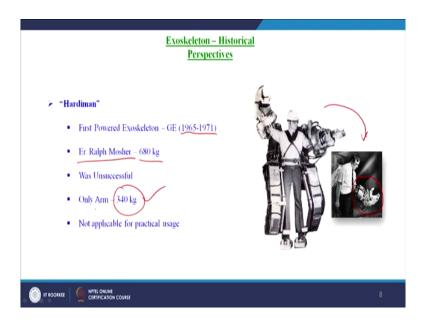
And, the very first practical exoskeleton has been developed by the general electric GE in the year between 1965 to 1971. It is the first powered exoskeleton and it is done by a group of engineers led by the engineer Ralph Mosher with the intention to lift up to 680 kilogram by this exoskeleton, but this task was unsuccessful by this Hardiman exoskeleton and later on they have focused to one arm exoskeleton that could able to successfully lift 340 kilogram,
