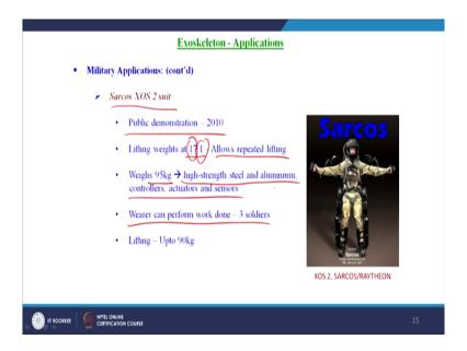
Now, coming to the second exoskeleton under the military application is Sarcos XOS 2 suit. It is a second generation suit of the Sarcos exoskeleton company and it is publicly demonstrated in the year 2010. The operator who is lifting the weight with Sarcos exoskeleton will feel the weight lifted in the ratio of 17 is to 1; that means, the actual weight is 17 times more than the perceived weight and also it allows the repeated lifting.
