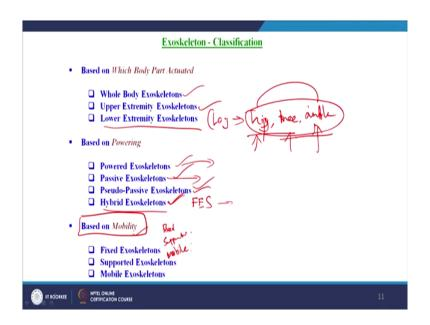
Now, coming to the classification of exoskeleton, first the classification is based on which part of the body is actuated. Accordingly it can be classified further into whole body exoskeleton if the full body is actuated and if the upper body, if the torso the neck and the arm are actuated then it is called upper extremity exoskeleton, and if the leg is actuated then it
