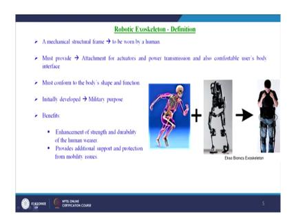
Now, coming to the definition of robotic exoskeleton, it is a mechanical structural frame to be worn by the human being for the sake of protection and support or power augmentation purpose. It must provide the exoskeleton structure must provide the attachment for actuators,
