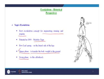
Now, coming to the historical perspectives of the exoskeleton – the first exoskeleton has been patented by Nicholas Yagn in the year 1890, and it was basically the conceptual of exoskeleton. So, this is for augmenting running and jogging. This is basically to bow leaf spring attached on the lateral surfaces or on the lateral sides of the legs two legs, so that in the stands face the exoskeleton spring is helpful to transfer the body weight to the ground.
