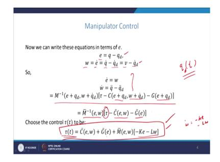
Now, according to the notation introduced earlier e is q minus q d and w, if you call is e dot we can write the same equation in the error form. So, e dot is equal to w we can give this notation and w dot is nothing, but e double dot. So, e double dot is from here it is q double dot minus q d double dot or in other words it is p dot minus q d double dot. So, we can get w dot is given by from the previous slide, we can write this one v dot is given by this last line.
