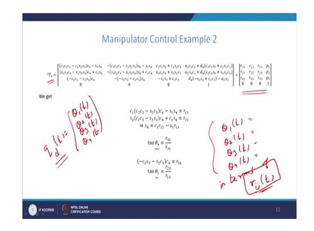
So, for performing this task we can design the problem in the following manner. So, firstly, the arm matrix 0 T 4 as we have seen in the inverse kinematics lecture, the 0 T 4 for this particular manipulator is given by this expression. So, if we know the 0 T 4 for each instant of
