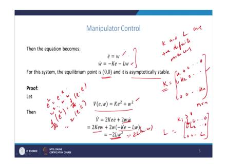
So, what we get the error system to be e dot is equal to w and w dot is minus K e minus L w, it is a very simple system of differential equation. And, we can easily verify that 0 0 is the equilibrium point. If, we equate the right hand side to 0, we will get w equal to 0 and putting it in the second equation, we get e equal to 0. Here, K and L are positive definite matrices.
