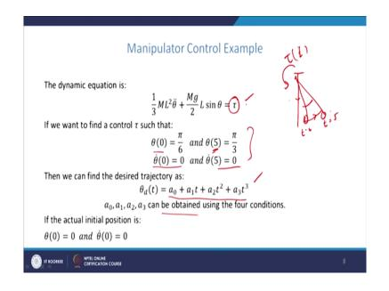
Then, we know that the equation is written in this particular form. We have already seen the dynamic equation of the single arm robot manipulator is written like this, where the torque access the control for this one. Now, we want to find the control of this pendulum, in this particular manner. That is a time T equal to 0 the angle is pi by 6, 30 degrees. And, a time t equal to 3 5 unit the angle is 60 degrees.
