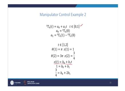
Similarly, we can calculate z of t as a function of time, and 0 T 4 as a function of time during the interval 0 to 1.
