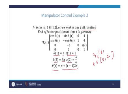
So, there are two conditions therefore, we can decide a trajectory as a polynomial of degree 2 degree 1. So, now, during the time 1 to 2, this crew makes 1 full rotation, that is angle 0 2 angle 2 pi it will make a rotation.
