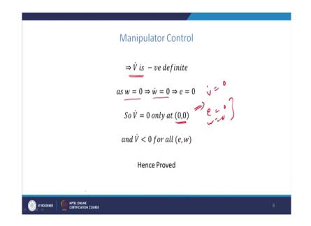
So, it is a negative definite value, even because when w is 0 automatically it will imply that e is also equal to 0, because when w equal to 0 w dot will be 0 and then both w and w dot or 0 from the equation given here, you can say that e is also equal to 0. Because, when w is 0 w dot is 0 K e is equal to 0 and K is positive definite therefore, the vector e is 0 vector.
