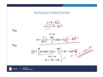
So, now after obtaining the desired trajectory as a function of time, we define the error actual angle is theta and desired angle is theta d as a function of time. These are all functions of time and w is e dot the derivative of e and that is nothing, but theta dot and theta desired dot the derivative. Now, we define the system in the form of error and it is derivative.
