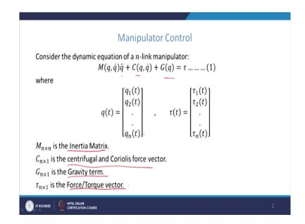
So, we have seen that it is written in the form of a system of second order differential equations, like M q double dot and C times C of q q dot plus G of q equal to tau, where q is
