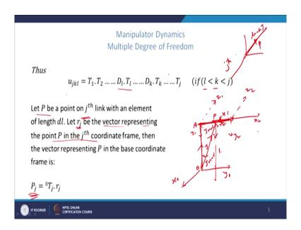
So, so for example, if you have ujkl it is if j l is less than k this D l T l will appear before D k T k or if l is greater than k then it will appear after this T k. So, in all the cases we can write ujkl notation to be the partial derivative. Now, let us assume that P be a point on the j th link
