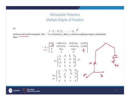
So, the last lecture we have seen how to write the dynamic equation of a two degree of freedom manipulator with uniformly distributed mass. So, here we consider a general n degree of freedom manipulator, whose arm matrix is written as 0 T n which is the product of
