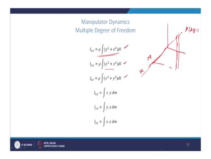
And, here also we can easily see the next slide we can see that i x x is nothing, but the inertia with respect to the X axis.
