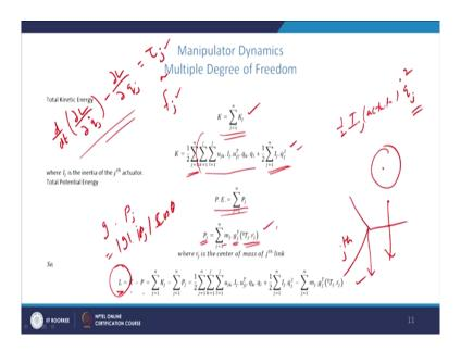
Now, the total kinetic energy is summation of all kinetic energies for the link 1 to n. So, we can simply write that the kinetic energy for the jth link is this and we are summing up all the so, it is j equal to 1 to n for all the links and the next two summation it gives the formula which we have given the kinetic energy of the jth link.
