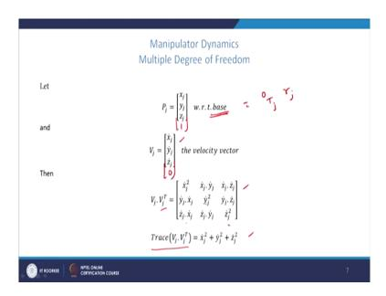
So, how to calculate that? We take the point P to be x j y j z j with respect to the base and V j is given by x its derivative is x j dot y j dot z j dot. And, V j is a column vector V j transpose is rho vector the same thing.
