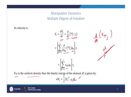
Now, the velocity of the same point means, we have to differentiate the vector P j with respect to time. So, d by dt of 0 T j into r j. So, we always keep it mind that r j is a fixed vector quantity and 0 T j is a function of q 1, q 2, up to q j here.
