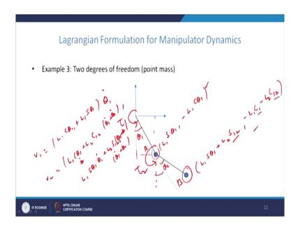
So, similarly here the double pendulum or a robot arm with two links here. So, the torque is applied at two joints here this is torque 1 and torque 2, both the joints are revolute joints here the.
