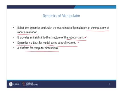
So, here so, the dynamics is nothing, but the equation of motion of the manipulator robot manipulator and the it provides the insight into the structure of the robot system. So, for example, if a robot is having n joints then there will be a system of n second order differential equation and the structure of the equation varies whether a particular joint is a revolute joint or prismatic joint etcetera.
