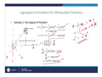
So, the first simplest case is the one arm manipulator. So, single arm manipulator or it is a controlled pendulum, we can say. So, where the torque is applied at the joint like this and the pendulum moves in the various directions. So, the motion of the pendulum we can analyze using this formula.
