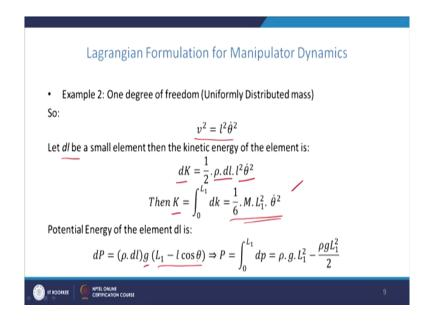
Now, if you take a small element of length dL on this pendulum so, at that point Q the velocity given by the velocity V square the modulus of the velocity vectors square is small 1 square theta dot square.
