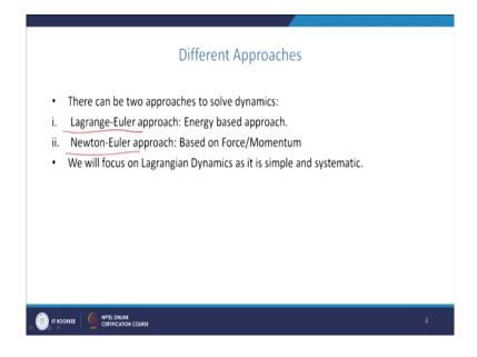
So, so to formulate the dynamic equation there are two approaches one is the Euler Lagrange approach which is energy based approach and another is the Newton Euler approach and it is based on the force and momentum of the manipulator. So, here in this lecture, we will concentrate on the Lagrange method; Euler Lagrange method.
