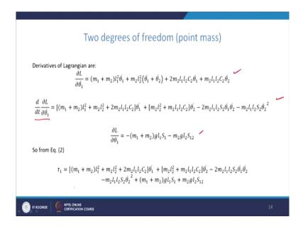
We have to calculate the del L by del theta 1 dot and then del L by del theta 2 dot for the second equation. So, first del L by del theta 1 dot directly we can differentiate with respect to theta 1 dot only. So, this term is to be differentiated, this is to be differentiated.
