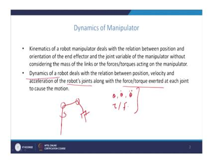
So, it will not take into account the mass or the force torque of exerted on the robot manipulators for causing a particular motion. So, for example, if you have the robot
