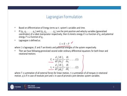
But another procedure is the Euler Lagrange method it is based on the Lagrangian L which is the difference between the kinetic energy and the potential energy of a body in motion. Any rigid body can be analyzed using this procedure in our case it is the robot manipulator.
