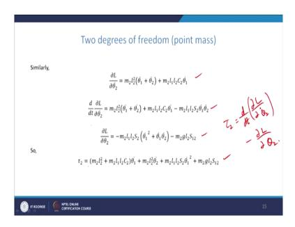
Similarly, for theta 2 del L by del theta dot is this and then its time derivative is given by this and del L by del theta 2 is given. So, we get the formula the torque 2 is d by dt of del L by del theta 2 dot minus del L by del theta 2. So, if you substitute these values, we will get the equation second equation tau 2.
