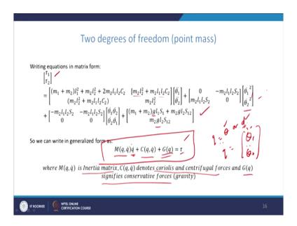
So, we observed that the equation of motion the tau 1 and tau 2 can be written in the matrix form like this combining the two equation. Here, the tau 1 equation is having components of theta 1 double dot. These are all theta 1 double dot and this is theta 2 double dot and remaining are theta 1 dot.
