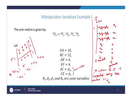
So, that we have seen in the previous lecture as the following. So, the J 6 cross n matrix in general; how it is calculated? It is calculated by the following formula; it is minus n x P y plus n y P x minus o x P y plus o y P x minus a x P y plus a y P x and n z del dot n, so n z, o z, a z. So, this is the first column. Similarly we can calculate the second column, if it is revolute joint. And if it is a prismatic joint we will get; n z, o z, a z, 0, 0, 0 if prismatic.
