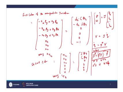
So, now let us calculate; so the first column of the manipulator Jacobian. So, it is actually given by the values minus n x P y plus n y P x minus o x P y plus o y P x and n z, o z, a z. So, this is using 0 T 4 columns at that particular values; so we can substitute here directly by seeing n x P y etcetera from the expression given here, 0 T 4. You can see that n x is cos of theta 1 minus theta 4 and P y is minus d 2 cos theta 1.
