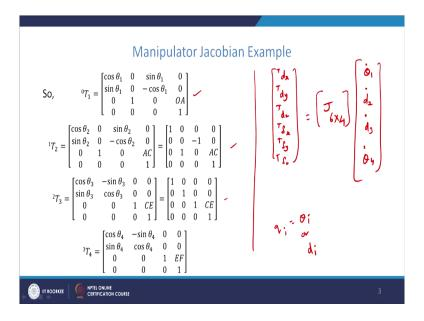
So, now by substituting the parameter values we can obtain 0 T 1 as given here 0 1 T 2; if you put i is equal to 2 we get 1 T 2 in the previous expression. And i equal to 3 will give 2 T 3 as given here etcetera. So, the four matrix; 0 T 1, 1 T 2, 2 T 3, 3 T 4 is obtained for the previous example in the by substituting the parameter values.
