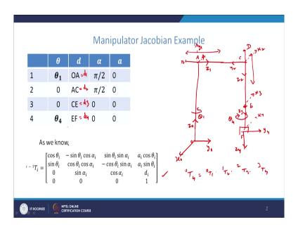
So, let us consider the robot manipulator shown in this figure; where the first joint is a revolute joint that is theta 1 and the second joint A is it is a prismatic joint, it slides in the forward and backward direction; the third joint C is also a prismatic joint moving up and the down; the fourth joint E is a revolute joint it is a rotational the angle is denoted by theta 4.
