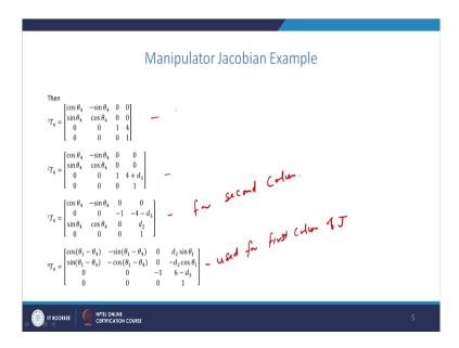
Now, 3 T 4 is given as it is for the parameter values. So, let us assume that the length is O A is 10, B C is 12, D E is 6, E F is 4 etcetera, so this values are given. And A C and C E these are the variables; because the joints are prismatic joints. So, substituting the values in this expression we get the values to be like this; the calculation of 3 T 4, 2 T 4, 1 T 4 and 0 T 4.
