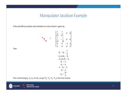
So, the Jacobian matrix is calculated at every instant of time; actually when the robot is moving to various position at a particular position what is the value of the Jacobian that can be calculated, because all this theta 1, d 2, d 3, theta 4 are varying. So, as they are changing what is the Jacobian matrix. So, at a particular instant of time; let us say the end effector is in this configuration.
