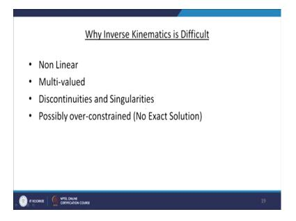
So, in general the inverse kinematic solution will be difficult if we have more complicated robot manipulators and it is multi-valued because to reach a particular position and orientation we can get several solutions and there may be singularities because if we give a particular x, y value the end-effector position, then angle does not exist for outside the range values. So, it means that the position x, y is outside the reach of the robot manipulator.
