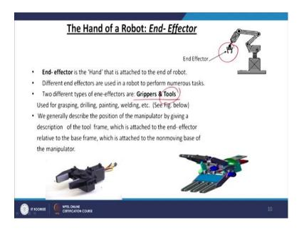
So, the hand of the robot manipulator is also called the end-effector. And, it is of two types; gripper and tools; the gripper is a machine with which has two fingers for example, like this or it can be like a human fingers or it can have simply the tool attached at the end-effector at the end of the robot manipulator that is also called a end-effector here.
