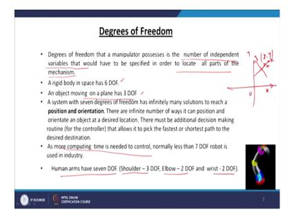
So, degree of freedom is the number of variables which is required to identify the parts of a robot manipulator. So, the number of independent variables that should be specified in order to locate all the parts of a robot manipulator. So, we know that a rigid body will have 6 degrees of freedom, 3 position variables and 3 rotation variables that is orientation variables.
