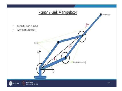
So, here we will see that a planar robot manipulator with three arms. So, here the first link has link  $l_1$ , second has  $l_2$  and third one has the link length  $l_3$ .
