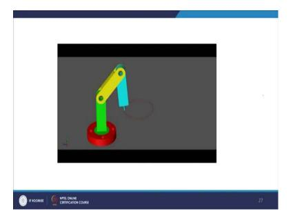
So, that is the three axis manipulator. So, the picture is depicted here and this video shows the exactly the same robot manipulator. The second link is rotating with respect to the axis perpendicular to this paper and the third link is rotating with respect to the axis parallel to the various axis of rotation and the base is rotating with respect to the axis which is vertical line.
