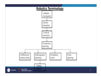
So, here the terminology are like this we have seen a roughly about a robot manipulator and the direct kinematics means how to write the position of the end-effector with respect to the position of the base of a robot manipulator. The equation to be developed so, that is using the DH algorithm.
