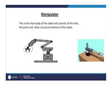
So, a manipulator is the body of the robot. So, here we can see the body and excluding the end-effector. The reference frame.
