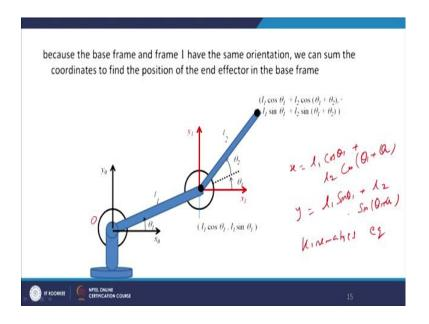
So, with respect to the origin O the x, y coordinates are given by this two formula and which is called the direct kinematics equation.
