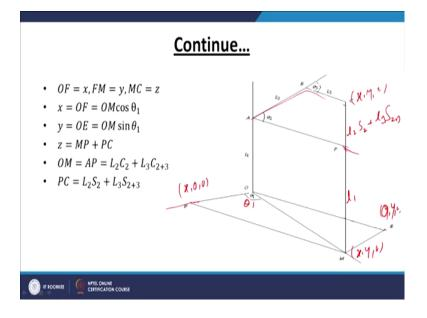
And, so, the inverse kinematics of the previous so, we see that the direct kinematic equation of this robot manipulator is given by the simple geometrical relation as in the equation 1, 2, 3.
