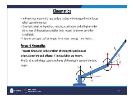
So, for a very simple robot manipulator all this calculations are very easy. We do not require the DH algorithm or anything just a simple geometry will give the kinematics equation and the inverse kinematic solution etcetera.
