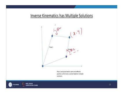
So, we can see that the link one is like this and if you extend it from here we measure the angle  $\theta_2$ . So, this is in the anticlockwise direction which is called the positive direction. So, if  $\theta_2$  is positive we get this configuration and if  $\theta_2$  is negative we get the other configuration.
