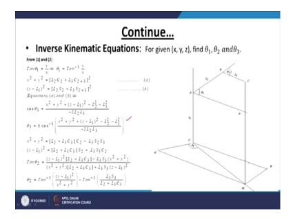
And, after writing the equation kinematics equation we can solve the inverse kinematics equation as we did it for the two link manipulator. So, we can easily see that the theta 2 is given by cos inverse of this expression.
