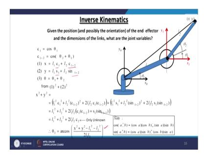
So, this is called the kinematics equation. Now, if  $\theta_1$  and  $\theta_2$  are given it is easy to find x and y. So, that is called direct kinematics, and if x and y are given find the value of  $\theta_1$  and  $\theta_2$  that is called the inverse kinematics solution of the problem. So, inverse kinematics can be easily solved by using simple manipulations mathematical manipulations like:
