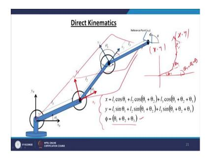
So, the solution the kinematics equation is similar to the previous one two link manipulator if the end-effector position is x, y you can write
