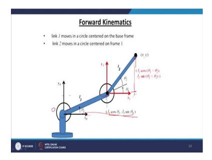
So, using this information and the information that the length of link 1 is  $l_1$  and the link 2 is  $l_2$  we can easily get the equation connecting x, y and the  $\theta_1$  and  $\theta_2$ . So, that is very simple to see here.
