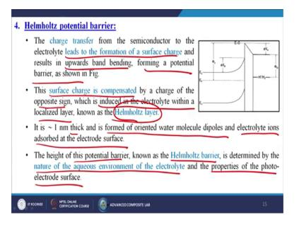
Next the fourth one is called the Helmholtz potential barrier. The charge transfer from the semiconductor to the electrolyte leads to the formation of a surface charge and results in upwards band bending forming a potential barrier as shown in this particular image. This surface charge is compensated by a charge of the opposite sign, which is induced in the electrolyte within a localized layer known as the Helmholtz layer basically.
