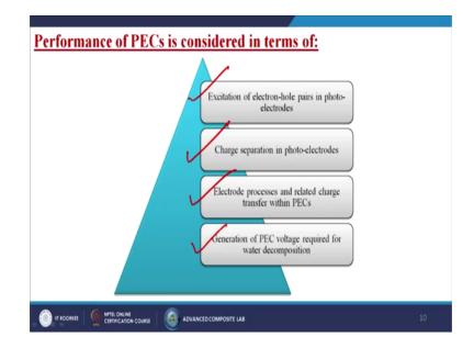
Now, what is the performance of PECs is considered in terms of excitations of electrons hole pairs in photo-electrodes, charge separation in photo-electrodes, electrode process and related charge transfer within PECs, and generation of PEC voltage required for the water decompositions. So, these all are the 4 different performance by which the total efficiency of this particular systems can exist.
