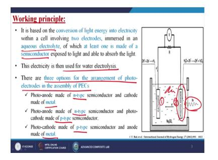
Now, what is the working principle? Basically, it is best on the conversion of the light energy into electricity within a cell involving two electrodes. So, you can see that that is the number 1 electrode which is acting as a cathode and another one is acting as a anode. So, basically, two electrodes we are using over here, immersed in an aqueous electrolyte.
