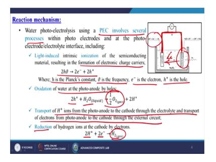
Then what is the reaction mechanism? So, what are photo electrolysis using a PEC involves several processes within photo-electrodes and at the photo-electrode or maybe the electrolyte interface including light induced intrinsic ionization of the semiconducting material resulting in the formation of electronic charge carriers which is happening in this particular case itself, when the sunlight or maybe the light is directly coming to the photo-electrode itself.
