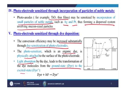
Next the fourth one is called the photo-electrode sensitized through incorporation of particles of noble metals. Photo-anodes for example, titanium dioxide thin films maybe sensitized by incorporation of small particles of the noble metals, such as silver or maybe the platinum or may be sometimes the both thus forming a disperse system involving micron sized particles. Now, the nanotechnology has come into the picture. So, people
