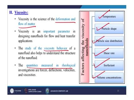
Next viscosity so, in this particular case viscosity is the science of deformations and the flow of matter right, this is a simple Layman description. So, viscosity is an important parameter in designing nanofluids for flow and heat transfer applications.
