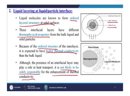
Next second one is the liquid layering at liquid particle interface. So, basically liquid molecules are known to form ordered layer structures at solid surfaces. These interfacial layers have different thermo physical properties from the bulk liquid and the solid particles. Because of the ordered structure of the nanolayer, it is expected to have higher thermal conductivity than the bulk liquid.
