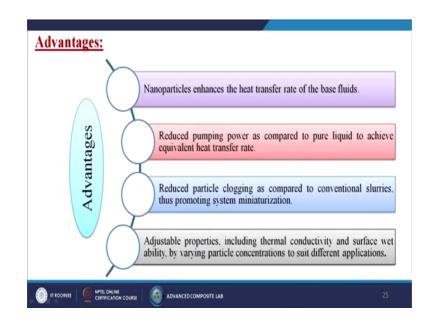
Then what are the advantages. So, basically nanoparticles enhance the heat transfer rate of the base fluids, till now we have discussed all this points. Second it is going to reduced pumping power as compared to pure liquid to achieve equivalent heat transfer rate, because it is consuming the more heat by applying the nanoparticles into the system. Third one it reduced particle clogging as compared to conventional slurries thus promoting system miniaturization.
