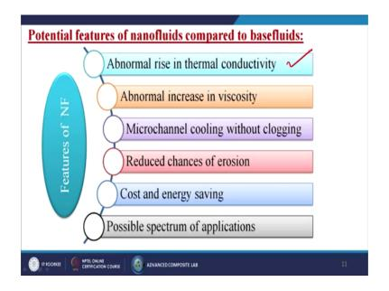
Now, what are the potential features of nanofluids compared to base fluids, first is that abnormal rise in thermal conductivity, abnormal increase in viscosity, microchannel cooling without clogging, reduced chances of erosions, cost and energy saving and the possible spectrum of applications. So, these all are the features for nanofluids.
