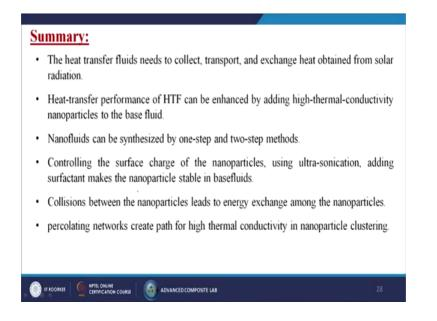
Nanofluids can be synthesized by one - step method or maybe the two - step method, controlling the surface charge of the nanoparticles, using ultra-sonications, adding surfactant makes the nanoparticle stable in base fluids also it will make a barrier in between the agglomerations of the nanoparticles.
