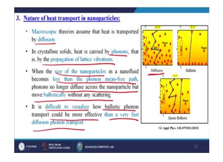
Next third one is called the nature of heat transport in the nanoparticles means which way the heat is transferring into the systems. Macroscopic theories assume that heat is transported by the diffusion method. Basically in crystalline solids, heat is carried by phonons, that is by the propagation of lattice vibrations. So, simple the vibration is taking place in between the phonons so, due to that vibration the heat is producing.
