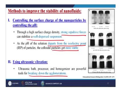
Now, how to improve the stability of the nanofluids so, there are several methods the first one is that controlling the surface charge of the nanoparticles by controlling the pH. So, basically through a high surface charge density, strong repulsive forces can stabilize
