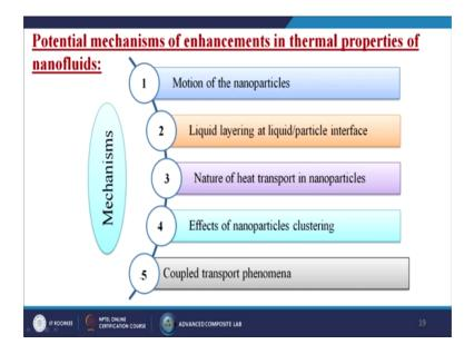
Now, what are the potential mechanisms of enhancement in thermal properties of the nanofluids. So, first is called the motion of the nanoparticles, because in the liquid systems you are having the nanoparticles so, movement of the nanoparticles inside the fluid.
