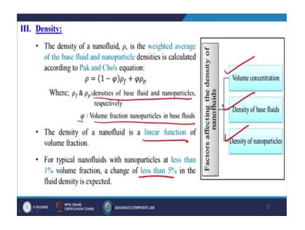
Next third one is called the density. So, the density of a nanofluid which is nothing, but the universal nomenclature rho is the weighted average of the base fluid and nanoparticles densities is calculated according to the Pak and Cho's equations. What is that particular equations, rho is equal to 1 minus sigma rho f plus sigma rho p.
